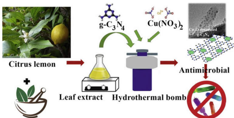
Fig. 2.7 Green synthesis of g\text{-C}_3\text{N}_4/\text{Cu}_2\text{O} via citrus leaves. (Reprinted with permission from Induja et al. (2019) copyright@2014 Elsevier Ltd. All rights reserved)
