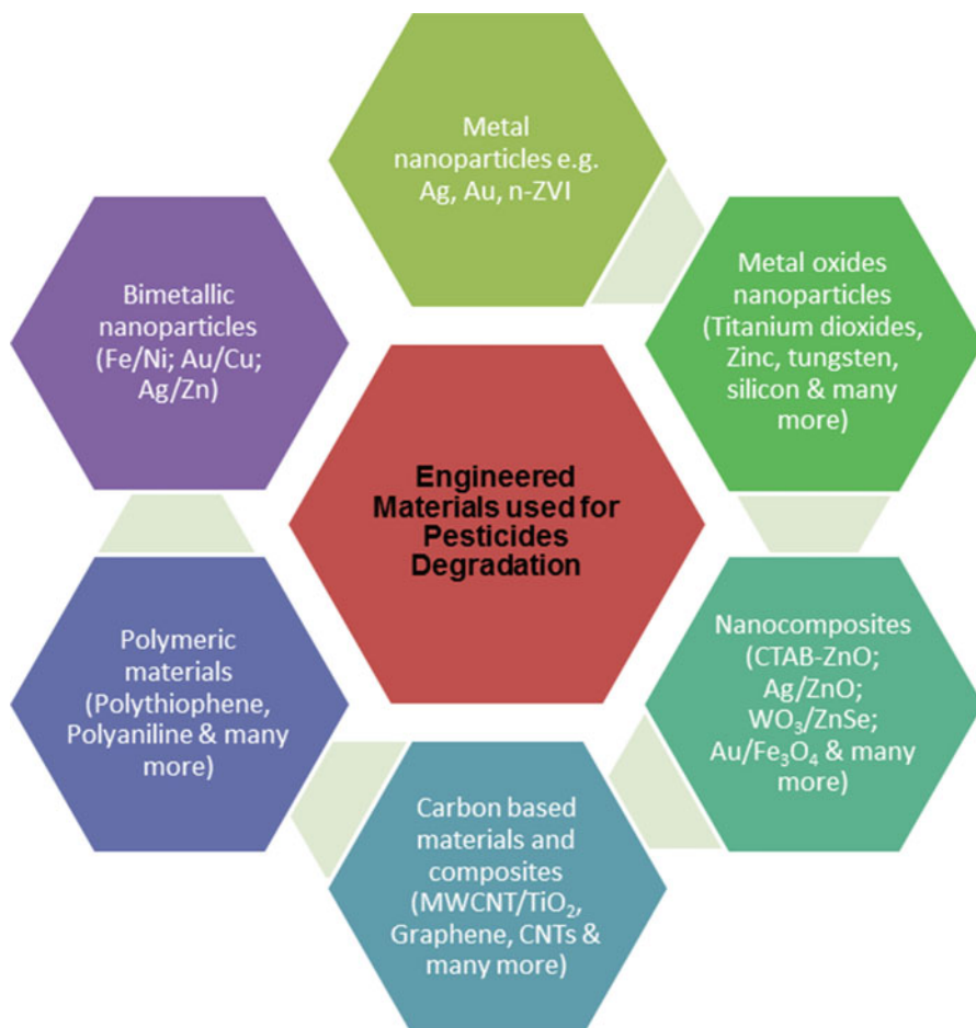
Fig. 7.2 Illustration of use of various types of engineered nanomaterials like metals, metal oxides, polymeric materials, nanocomposites for pesticides degradation from water and soil
