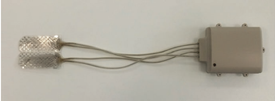
Fig. 3 The clinical-grade wireless neuroprosthesis with a 128-contact grid, 4 connecting cables, and the wireless case providing wireless ECoG transmission and DCS
