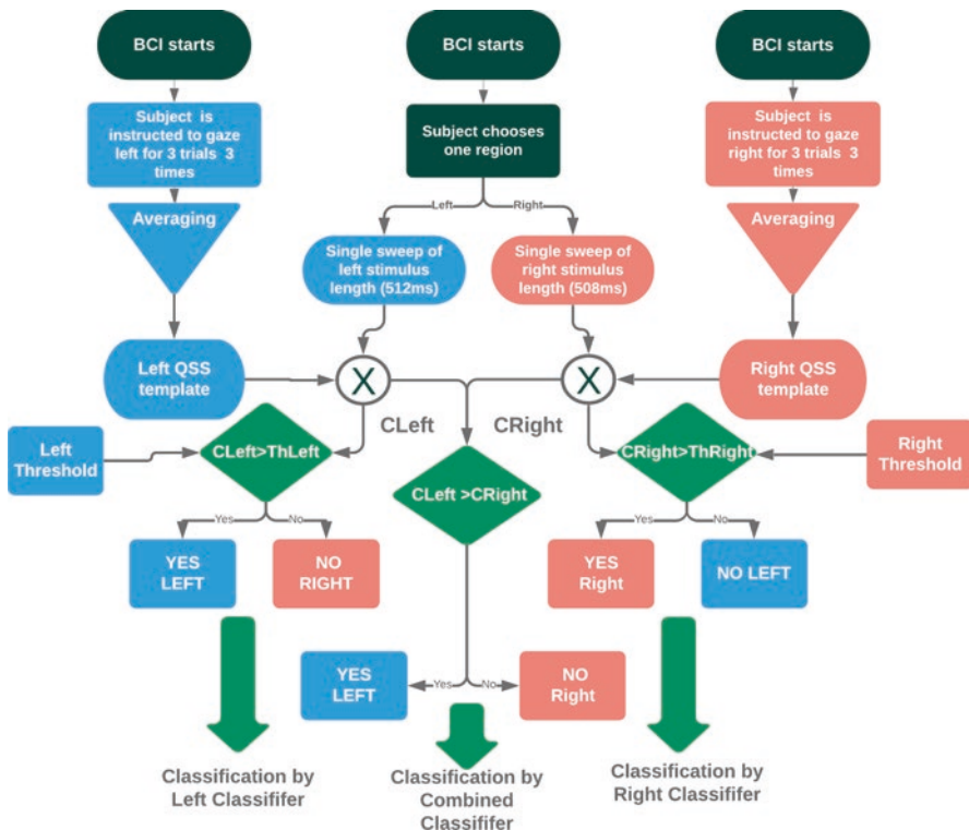
Fig. 3 Three types of classification and command/target detection processes based on 10rps left and right QSS signals type are shown using two template comparison
