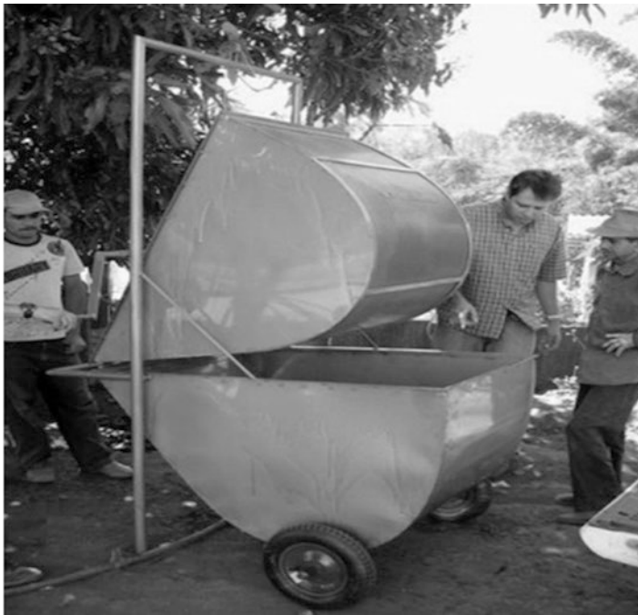
Fig. 1.7 Mobile coffee washer with tilting system to unload high density coffee beans. Source: Silva et al. (2014)
