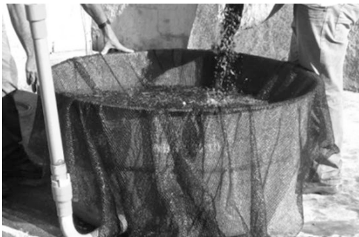
Fig. 1.8 Rustic homemade coffee washer using water box and shade screen to separate the high-density coffee. Source: Silva et al. (2014)
