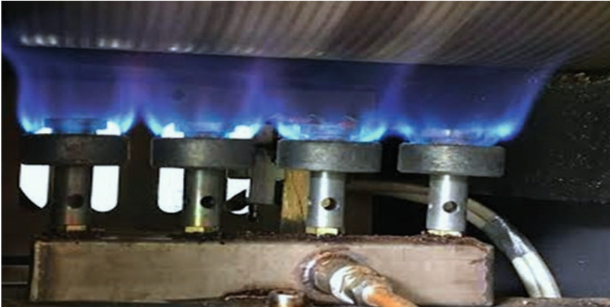
Fig. 7.2 Perforated wall roaster, flame burner image. Source: Authors
