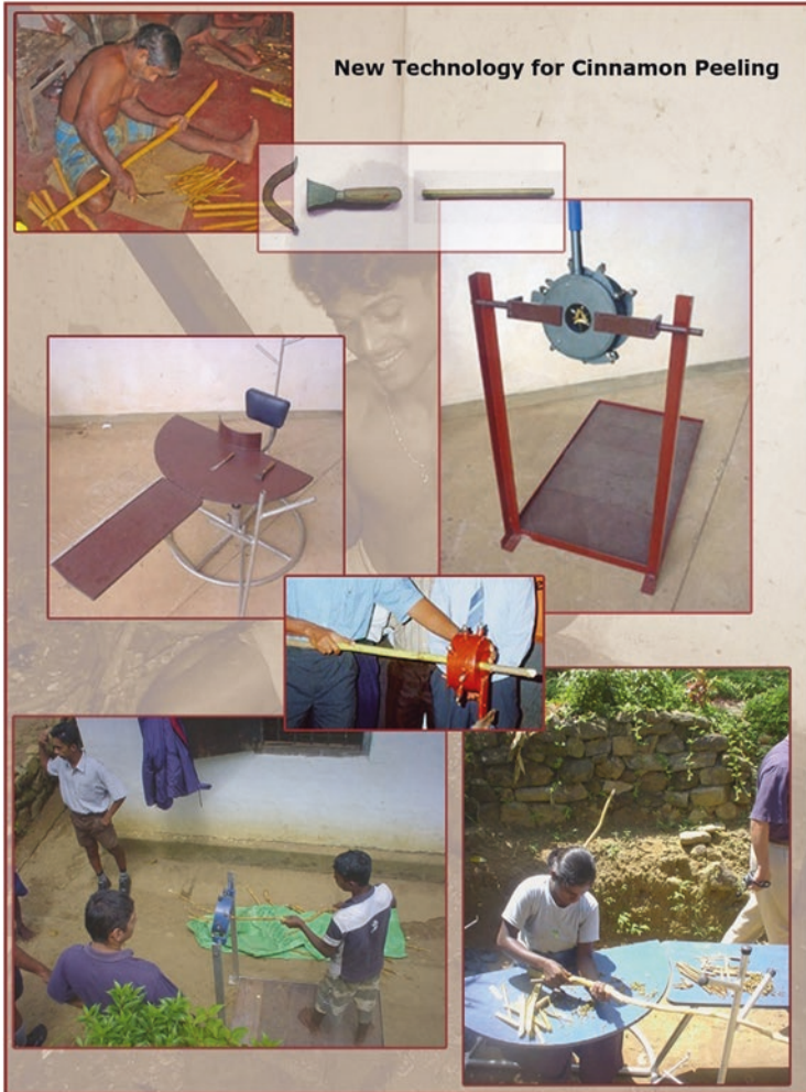
Fig. 9.10 Demonstration of technology shift in cinnamon peeling industry from floor operations to table operation (Weerasinghe 2011).
