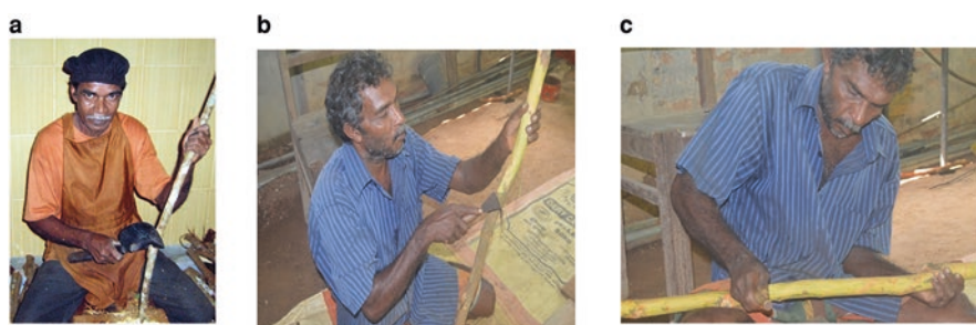
Fig. 9.3 (a) Removing knots with “ Keththa ”. (b) Scraping with “ Koketta ”. (c) Rubbing with a brass rod
