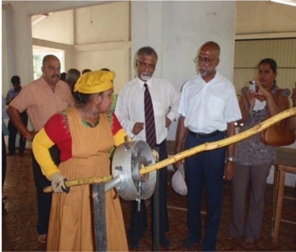
Fig. 9.12 RUWEKA-PG with the stand and cam mechanism to insert sticks
