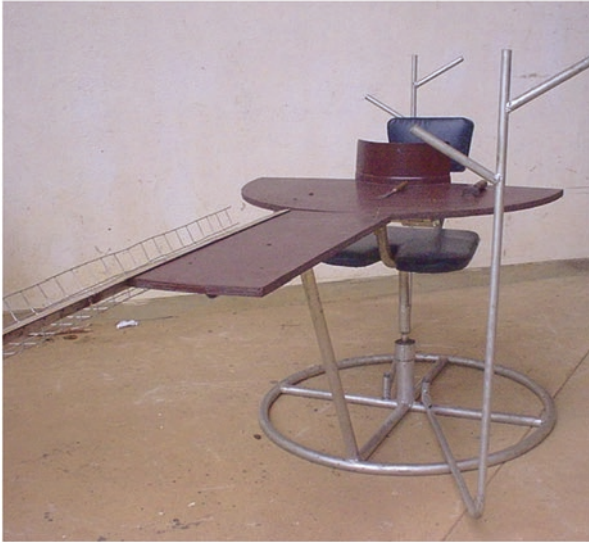
Fig. 9.14 Cinnamon processing bench introduced by Department of Agricultural Engineering, University of Ruhuna. Industrial Design 7628. (Weerasinghe and Pushpitha 2005b)
