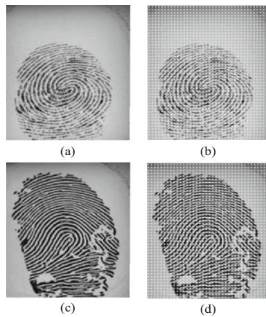
Fig. 2. True, fake fingerprints and their visualizations using HOG. (a) True fingerprint. (b) True fingerprint visualization. (c) Fake fingerprint. (d) Fake fingerprint visualization.
