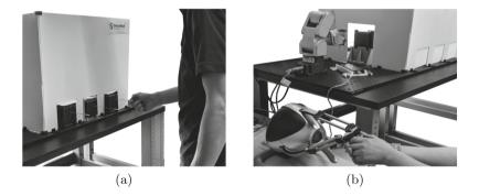
Fig. 5. The two stages of the user trials. (a) The test participant would first insert the needle by hand to determine the depth of the cancer layer in three unique phantoms. (b) The participant would then determine the depths using haptic feedback in the teleoperated scenario.
