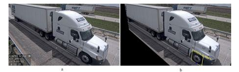
Fig. 3. (a) original image, (b) detected tire-road contact point in the perspective image.
