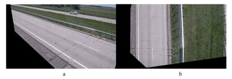
**Fig. 5.** (a) Original image with perspective distortion, White lane markings converge at a finite point. (b) Homography-based transformation from perspective to a scaled orthogonal image – a bird's eye view – non vehicle image.
