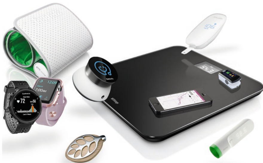
Fig. 6.1 An overview of commonly used smart sensors, including smart-watches with heart-rate and activity tracking, an activity tracking jewel, a blood pressure cuff, stethoscope, scales, glucose meter, pulse-oximeter, and body thermometer, all of which allow for at-home health monitoring
