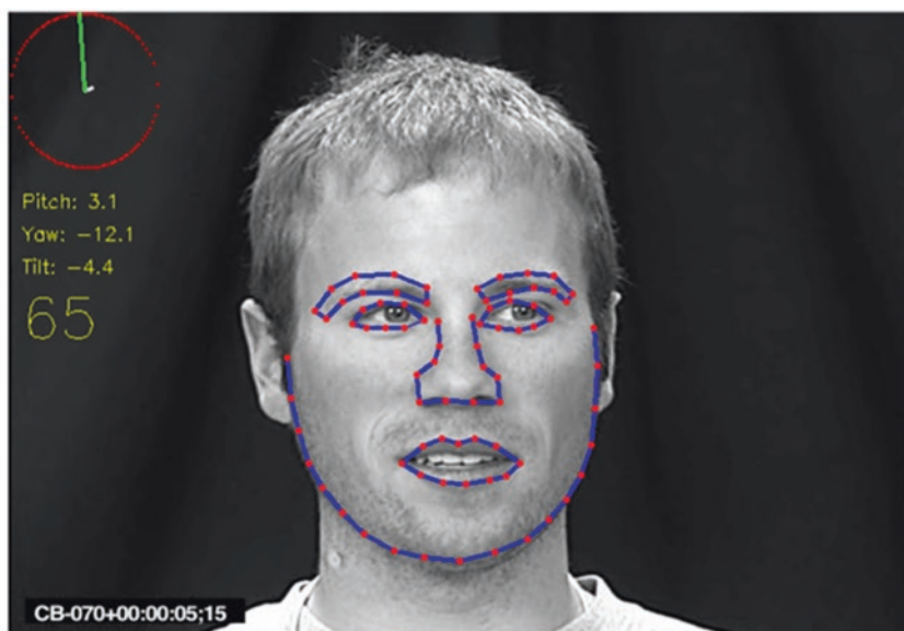
Sample frame showing tracking of the 79 facial landmarks. The circle in the upper left corner depicts the estimated 3D vector of the head pose. Underneath it are the estimated values of the pitch, yaw and tilt angles of the head
