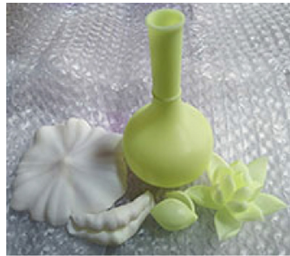
Fig. 2. The porcelain and lotus produced through AM
