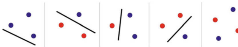
Fig. 2 A 2D-line can separate a set of three points in all possible ways, whereas there exists a formation of four points which cannot be achieved by a separating 2D-line. Thus, the VC-dimension of a 2D-line equals h = 3
