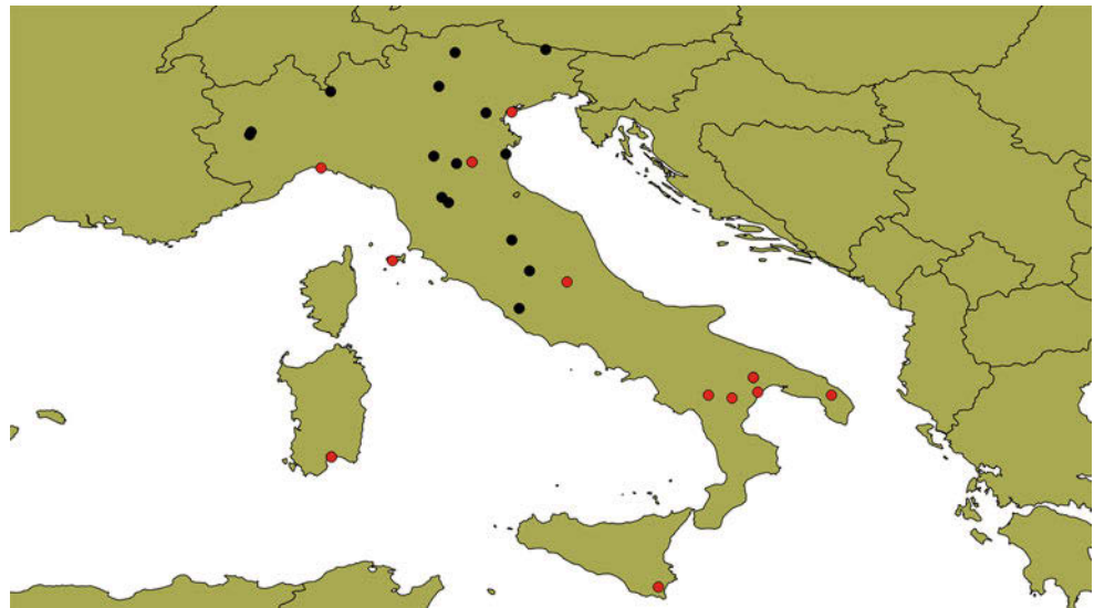
Fig. 1 GNSS Reference frame network currently powered by ASI (in red) and Italian EPN – EUREF network (in black)
