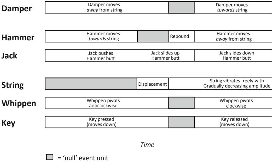
Fig. 2. Event unit analysis for piano mechanism operation (initial version). The time course of the mechanism’s operation can be divided into three successive stages – (1) Strike, (2) Rebound, and (3) Reset.
