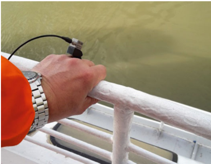
Fig. 2 The triaxial accelerometer in finger support
