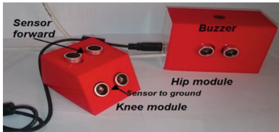
Fig. 4 Modules construction with the three sensors and buzzer [7]
