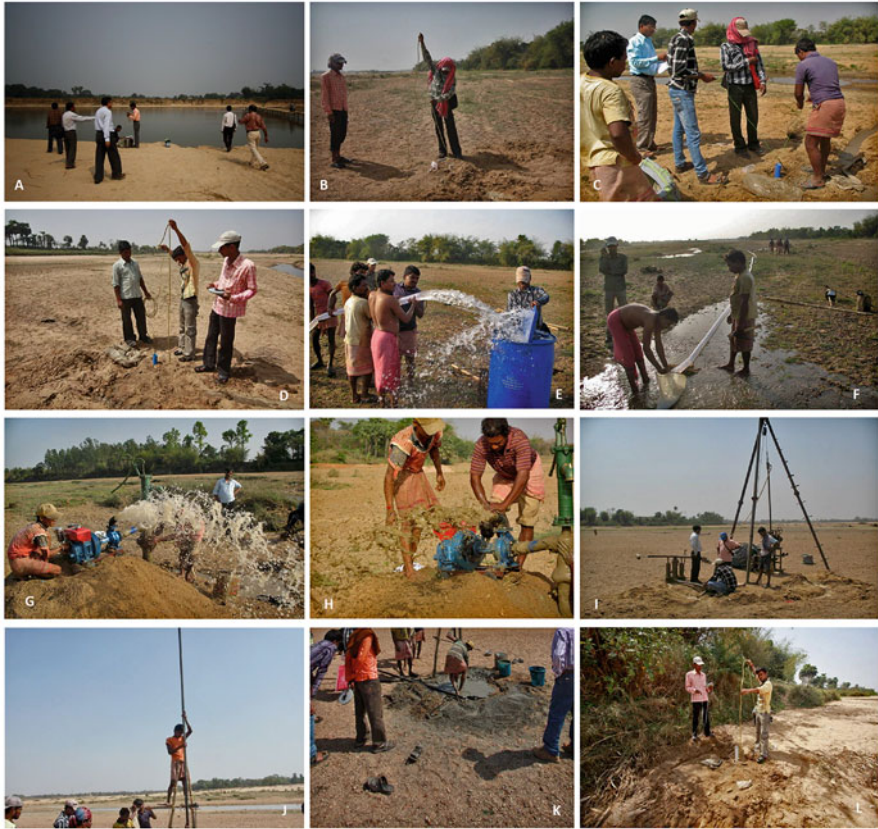
Fig. 9.5 Photographs depicting different field activities relating to insertion of bore-well for studying pumping cycle (A–D); Geological, geomorphological and lithological assessment of different fresh water riverine beds of Bankura and Purulia , Districts of West Bengal; (E to G) Extraction and quantification of subsurface and ground water with the help of bore wells and test wells to generate data for the evaluation of draw-downs; (H to L) Field activities pertaining to the installation of bore wells and test wells at specified site maintaining requisite distances based on the lithological assessment
