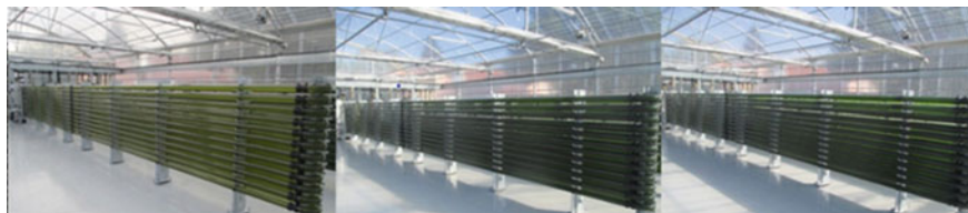
Fig. 3.3 Tubular reactor system for growing metabolically engineered Synechocystis sp PCC6803 viewed at various stages of cyanobacterial growth. The darkening colour indicates growth with time
