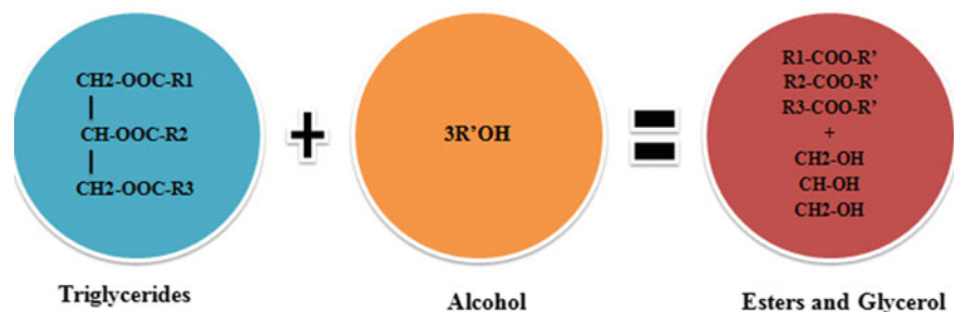
Fig. 15.4 Reaction showing the transesterification process (Parawira 2010)
