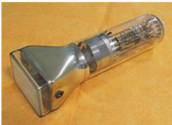
Fig. 1.14 Early oscilloscopes used CRT's to display waveforms. (Wikipedia)
