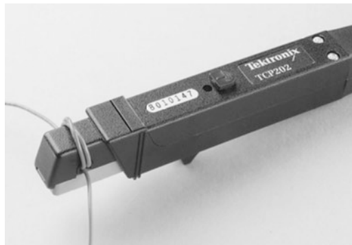
Fig. 2.29 Tektronix current probe. A technique for multiplying a weak signal is shown. Two or more turns are coiled, so they all pass through the jaws. This multiplies the current by the number of turns. The amount of current as measured by the oscilloscope must then be divided by the number of turns to arrive at the correct figure. (Tektronix)
