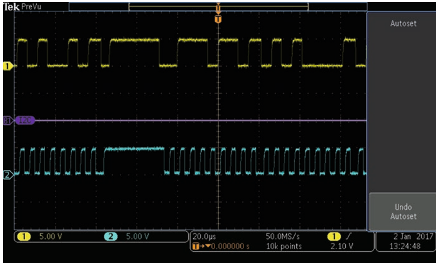
Fig. 6.17 I 2 C signals displayed in Tektronix MDO3000 series oscilloscope. (Tektronix)
