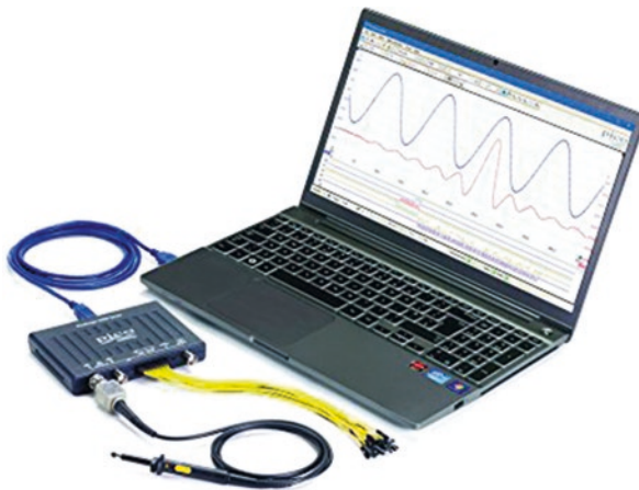
Fig. 9.1 The sine wave is a very basic waveform found throughout nature and in human-made machinery and electronic equipment. It occurs in mathematics, physics, engineering, signal processing, and elsewhere. Plotted on a graph where the vertical Y -axis represents volts and the horizontal X -axis represents time as in the oscilloscope's time-domain mode, the sine wave appears as a smooth periodic curve. All the power is at a single frequency, and it is free of harmonics. The curve has a pleasing appearance because of its symmetry, but the sound can be unpleasant because at moderate volume it tends to overload the auditory receptors at a single frequency. (Author's screenshot)
