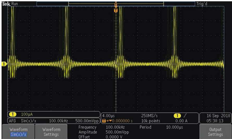
Fig. 9.7 The \sin(x)/x provides a ringing pulse useful for testing circuits with inductance. A sharp single pulse will have ringing with an inductive circuit where the higher frequency components are cutoff. This function simulates that behavior. (Author’s screenshot)
