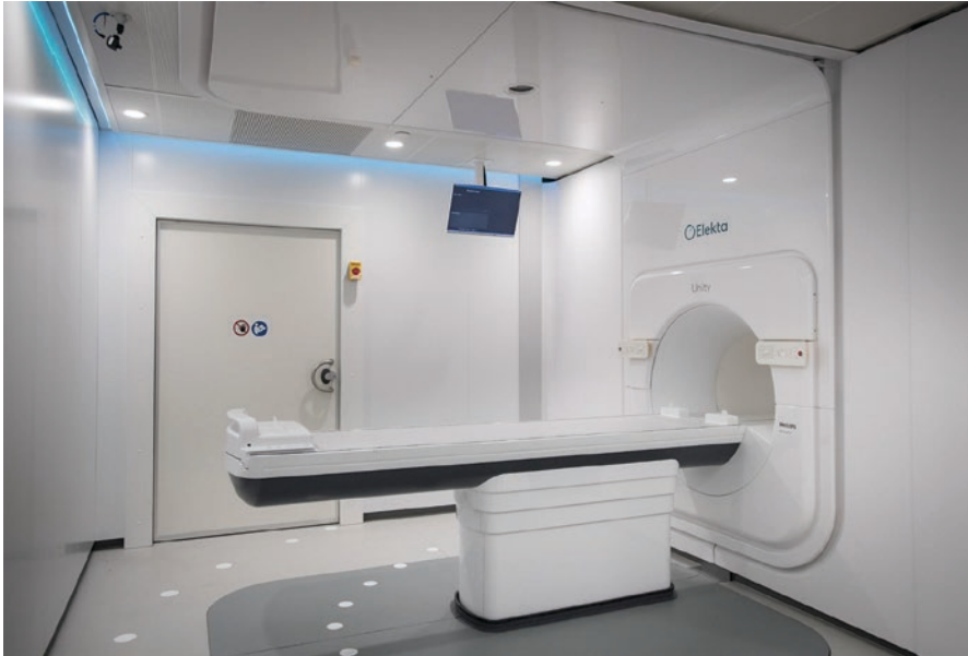
Fig. 46.4 MR-LINAC combines high resolution magnetic resonance imaging with a linear accelerator into a single machine. Photo Courtesy Sunnybrook Health Sciences Center Department of Radiation Oncology, Toronto, Canada
