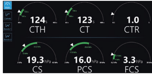
Fig. 41.3 Dials view screens used on the Quantra Hemostasis Analyzer (QPlus). Numerical results of specific parameters are displayed relative to a reference range (green segment on the dial)
