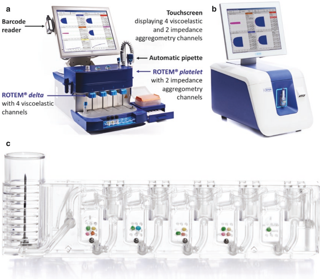
Fig. 18.1 (a) ROTEM® delta device (thromboelastometry) plus ROTEM® platelet module (whole blood impedance aggregometry), (b) ROTEM® sigma device and (c) ROTEM® sigma cartridge. (Courtesy of Klaus Görlinger, Tem Innovations)
