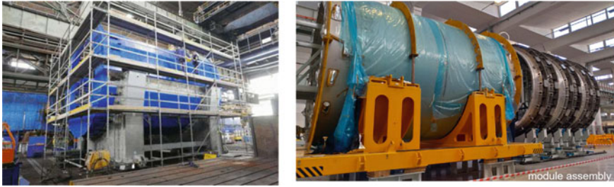
Fig. 79.3 Left: The yoke of the MPD magnet. Right: The MPD magnet solenoid
