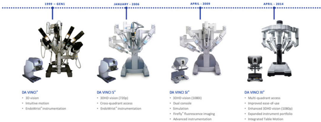
Fig. 59.4 Evolution of the da Vinci® Surgical System (with permissions from Intuitive Surgical, Inc)
