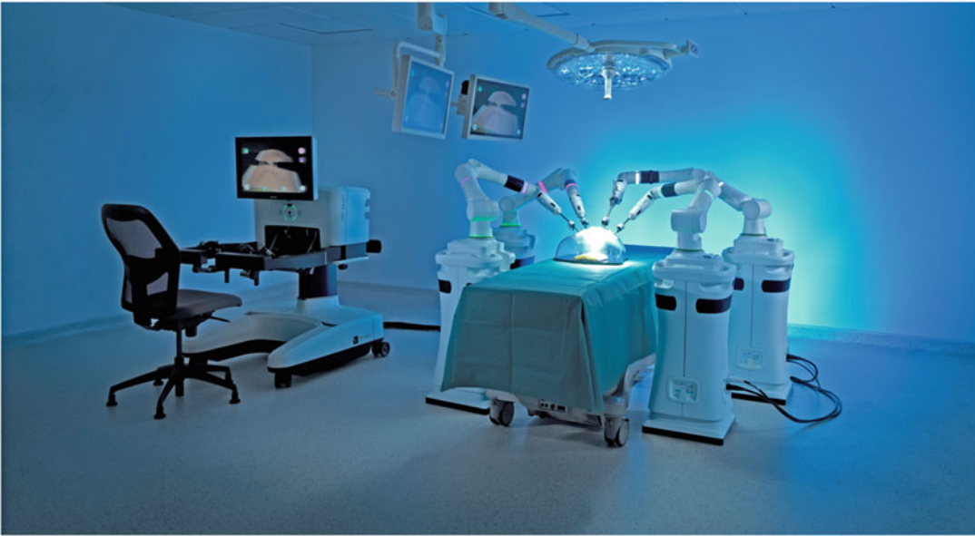
Fig. 59.16 Versius™ robotic system setup in the operating room (with permission from CMR)
