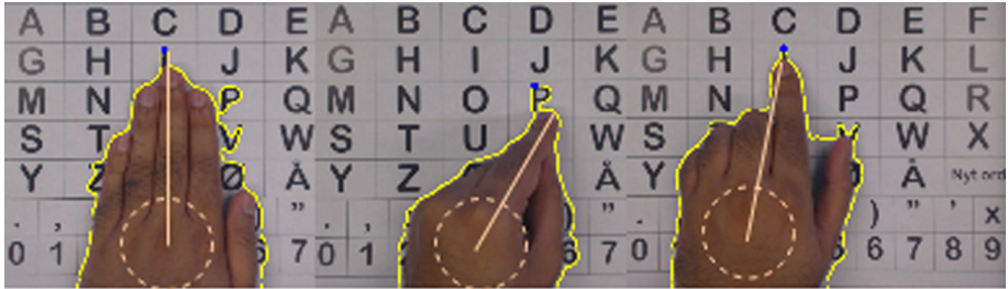
Fig. 4. Identification of a pointing finger by measuring the maximum distance from center of the palm to the fingers
