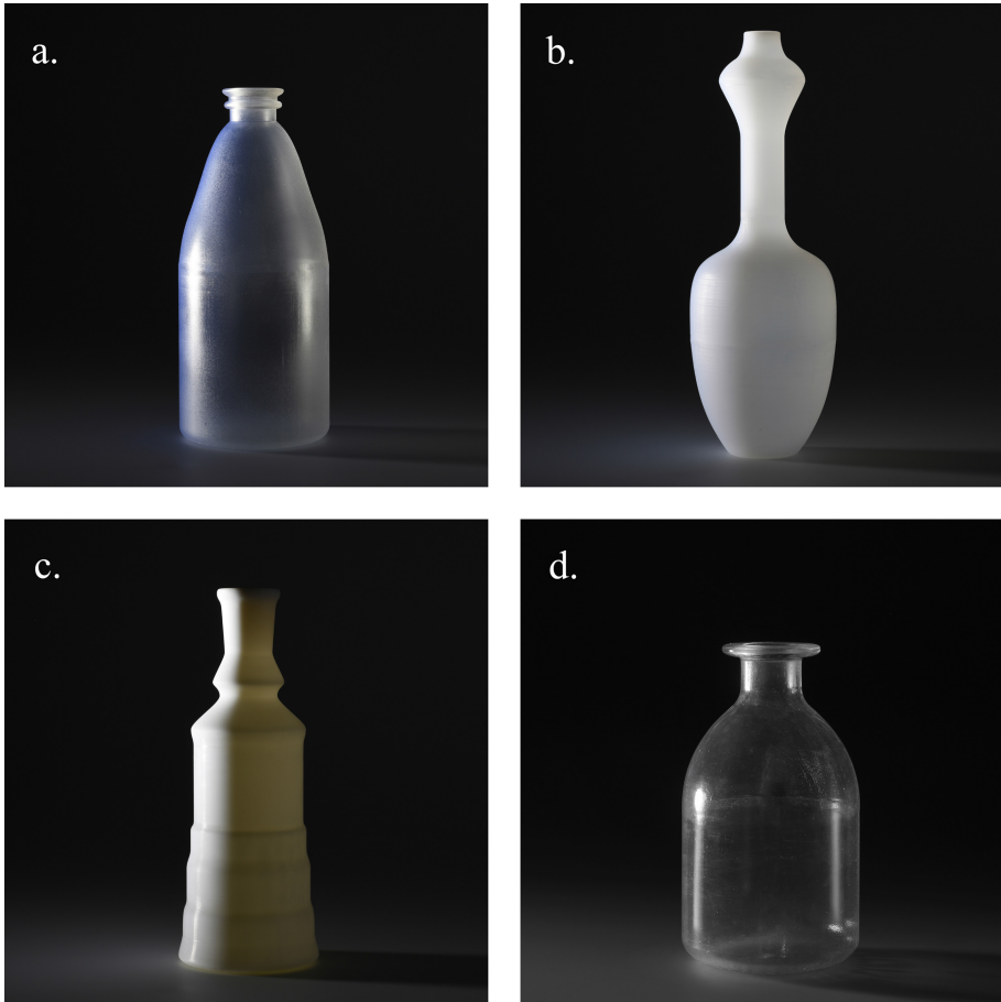
Fig. 10. 3D print of generated bottles using a. plausible shape representation, b. semantic shape representation, c. personal taste in shape representation, and d. democratized shape representation
