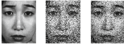
Fig. 7. Original image (left) and image with a Gaussian noise (middle) and Salt-and-Pepper noise (right) of 0.2 standard deviation
