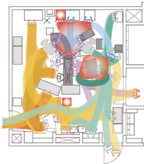
Fig. 13.1 Architectural flow diagram. Architectural plan indicating composite staff movement during the operative phase of observed procedures. The personnel are identified by a specific color (anesthesiologists are denoted in blue , surgeons in purple , nurses in tan , and perfusionists in green ). Each representation of a person indicates locations they have traveled, not the total number of people involved in the surgery. The density of the line color indicates the magnitude of movement within the time period studied. Red zones indicate areas with a high density of flow disruptions. Used with permission. (Palmer et al. [8])
