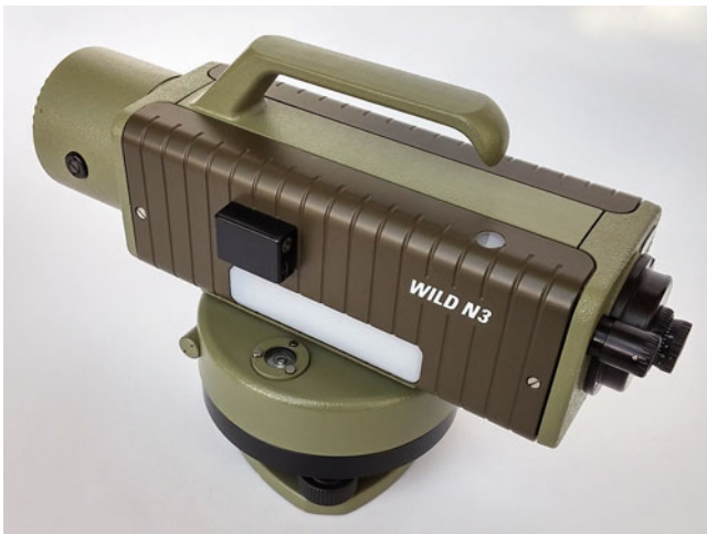
Fig. 11.17 Tilting level: the Wild N3 (courtesy of Trimble)
