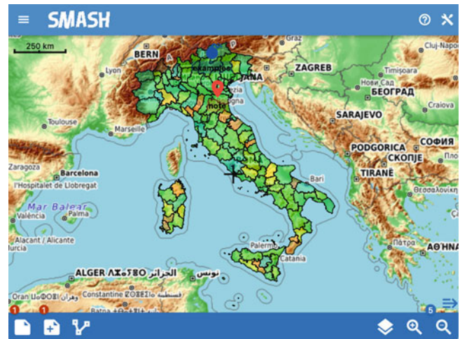
Fig. 30.15 The main view of S.M.A.S.H. visualizing a PostGIS polygon layer styled using OGC SLD theming
