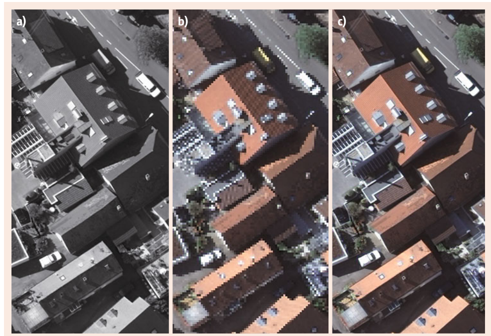
Fig. 9.6 The concept of pansharpening to increase the spatial resolution of color imagery. (a) High-resolution PAN, (b) RGB low resolution, and (c) RGB after pansharpening. Courtesy of ifp-Stuttgart
