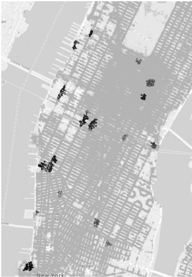
Fig. 5.4 Spatio-temporal clustering (DBSCAN) of ridesharing drop off locations in Midtown Manhattan. This identified clusters (darker points in the figure) where many drop offs occurred in a similar place and time and the minimal cluster size is 15 events
