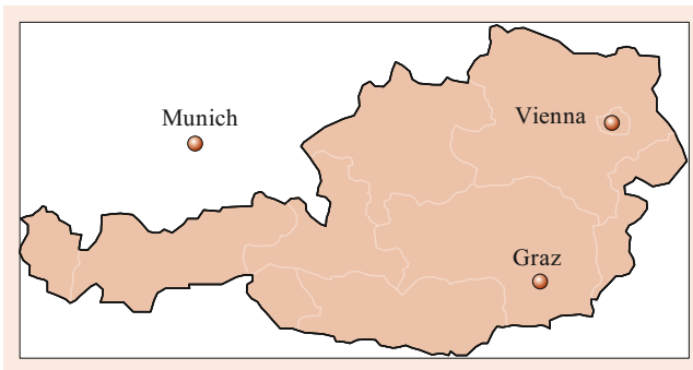
Fig. 6.21 A range query retrieves a false hit that will be discarded in a subsequent detailed point-in-polygon test
