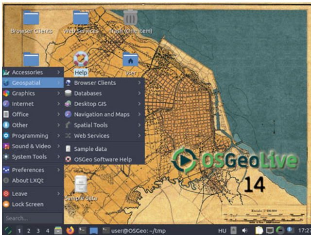
Fig. 30.24 Overview of the user menus for geospatial FOSS tools in the OSGeoLive 14.0 desktop environment, comprising varieties of geospatial browser clients, databases, desktop GIS, navigation and maps, spatial tools, and map services
