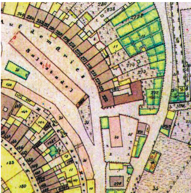
Fig. 20.6 Early example of a multipurpose cadastre containing buildings, land use information, and addresses
