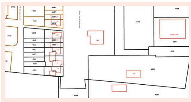
Fig. 20.26 Cadastral map of The Netherlands; cadastral boundaries and parcel numbers ( black ); provisional boundaries ( brown ); contours of buildings ( ground level ) in red ; house numbers in red
