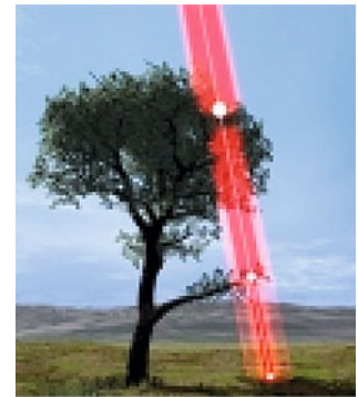
Fig. 9.13 Principle of multiple echoes from a laser signal. After [12], courtesy of the author
