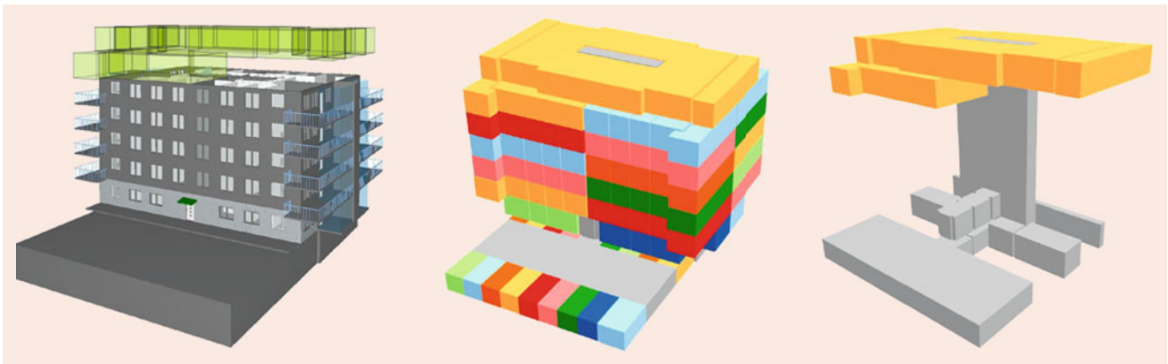
Fig. 20.29 First results of BIM Legal: extracting legal spaces using the IFC data model
