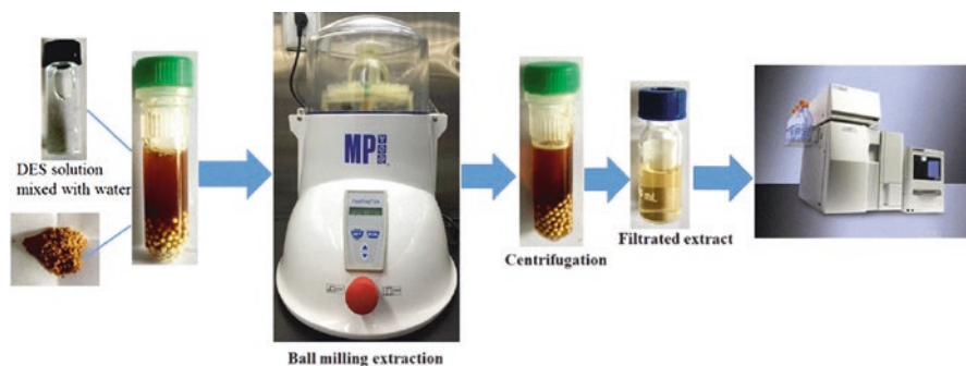
Fig. 6.9 Ball mill-assisted deep eutectic solvent-based extraction of tanshinones from Salvia miltiorrhiza Bunge . This method can induce an optimized motion to disrupt cells through the multidirectional, simultaneous beating of specialized beads on the sample. This leads to a full release of intracellular products into the deep eutectic solvent (DES). (Figure reprinted with permission from Wang et al. 2016)
