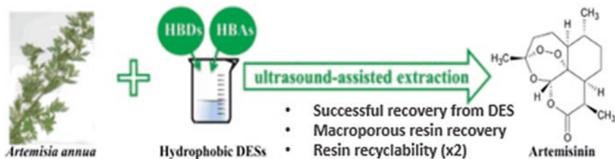
Fig. 5.6 Simplistic representation of extraction procedure to remove artemisinin from Artemisia annua leaves. 1:4 methyltrioctylammonium chloride/1-butanol gave the best extraction efficiency. (Reprinted with permissions from Cao et al. 2017b. Copyright (2017) American Chemical Society)
