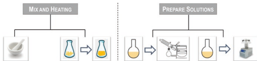
Fig. 3.4 Different methods described for the preparation of therapeutic deep eutectic systems (THEDES). In the mix and heating method, it is described that a mortar and a pestle could be used or otherwise it is possible to mix the compounds and by heating and stirring form a deep eutectic system. Other methods that have been reported are the preparation of solutions of different components and then evaporating the solvent or freeze-dried and a deep eutectic solvent (DES) is obtained
