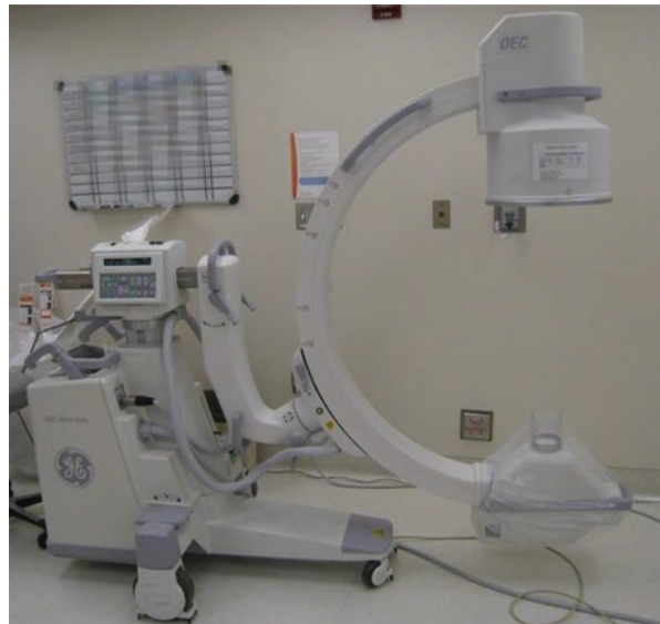
Fig. 2.2 The portable C-arm of a mobile fluoroscopic imaging system. The radiographer has to manually position the C-arm over the area of intervention
