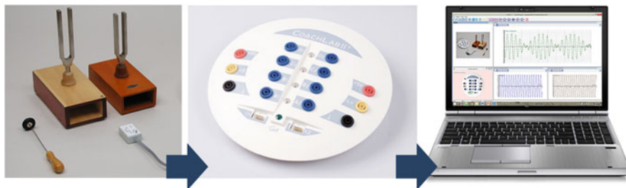
Fig. 12.1 Diagram of the tool for data logging with sensors (including sensor, interface and computer with dedicated software)
