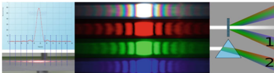
Fig. 19.3 Different dispersive phenomena: diffraction (left) and centre and dispersion (right) are used to highlight the chromatic structure of light. The colour turns out to be a parameter upon which such phenomena depend on
