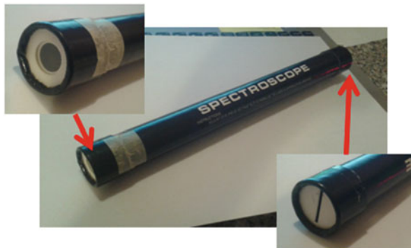
Fig. 19.2 A simple spectroscope: the slit allows light to enter the instruments, and the grating decomposes it in its colours
