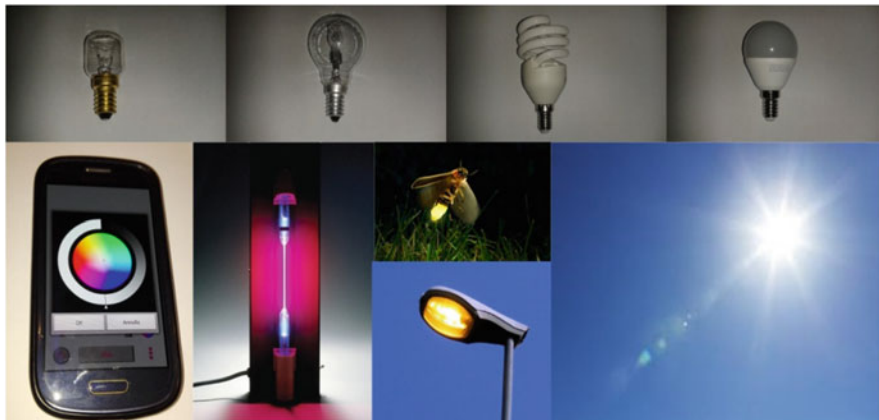
Fig. 19.1 Different kinds of lamps are presented in the path: incandescent, halogen, fluorescent, white and coloured LEDs, gas discharge. A reflection is also stimulated on the existence of natural mechanisms to emit light (thermonuclear reactions in stars, bioluminescence in animals) as well as artificial ones. A light source is thus seen as a system able to convert a form of energy in radiant energy, i.e. light
