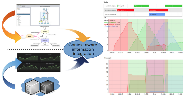
Fig. 4. The basic idea of the cross-context workflow execution analyser, and its output. In the right side of Fig. 4, user can interactively check the workflow processes (from the provenance), and check the system resource information (e.g. CPU and network).
