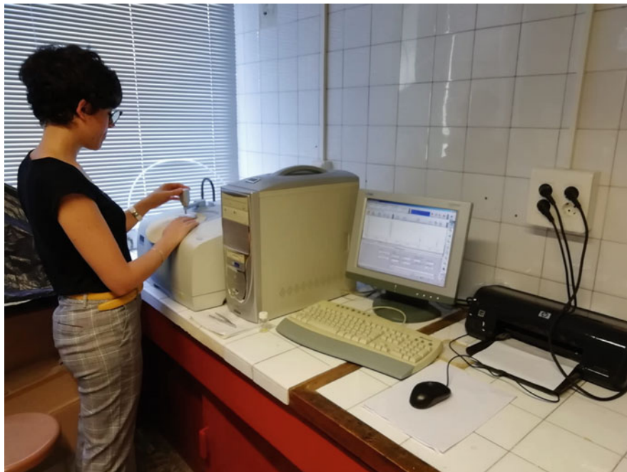
Fig. 1.2 Analysis of microplastics in Fourier transform infrared spectroscopy equipment, in order to find out their chemical composition
