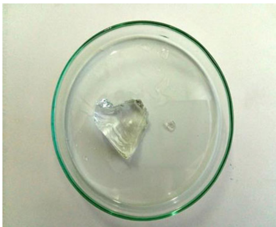
Fig. 7 The swelling capacity of the hydrolyzed hydrogel D-PAA-0.4-10. Swollen hydrogel— left ; the dried hydrogel— right
