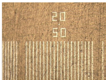
(a) Photolithographic pattern formed on nickel plated PTFE
