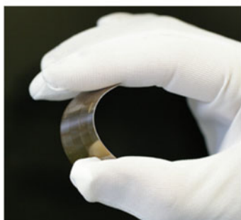
(b) Confirmation of the flexibility of PTFE having a photolithographic pattern formed thereon
