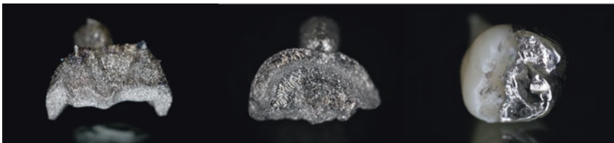
Fig. 30 3D printed chromium-cobalt onlay restoration. Occlusal surface (L), intaglio surface (C), and onlay cemented onto extracted tooth (R)
