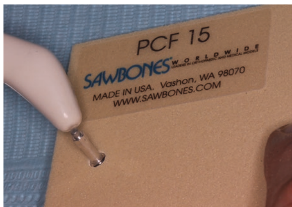
Fig. 7 Implants positioned into polyurethane foam blocks in 20 PCF corresponding to D2 bone density
