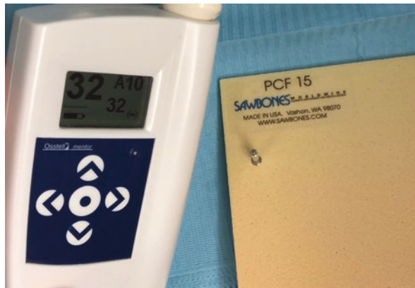
Fig. 6 Implant insertion. The insertion torque (IT, N cm) peaks indicated the force of the maximum clockwise movement of the dental fixture positioned into the material
