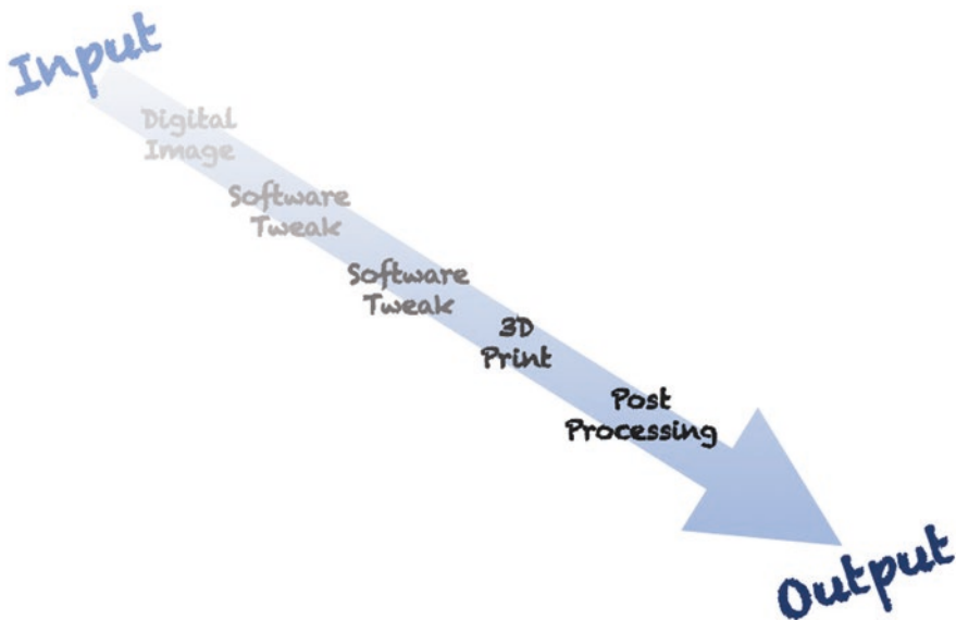
Fig. 7 Diagrammatic representation of the digital workflow associated with 3D printing
