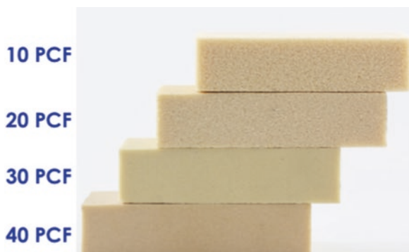
Fig. 1 Polyurethane blocks in different densities. 10 PCF, similar to D3 bone quality; 20 PCF, corresponding to D2 bone; and 30–40 PCF density, similar to D1 bone
