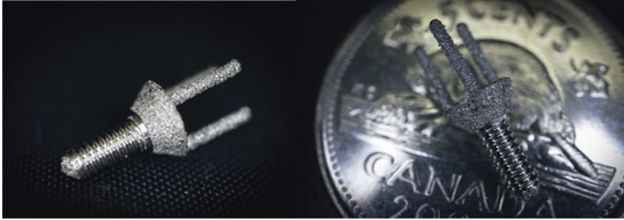
Fig. 29 3D printed novel dental implant abutment in titanium alloy. Final hybrid manufacturing abutment (L) and proportion to Canadian nickel for scale (R)
