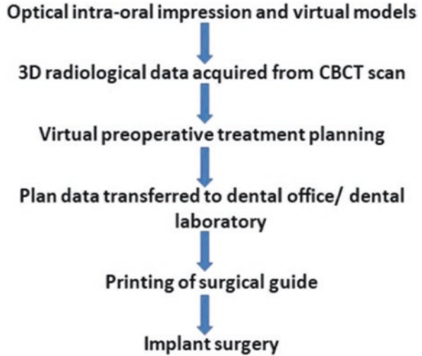
Fig. 2 Modified workflow involved in computer-generated surgical guide and computer-guided implant surgery
