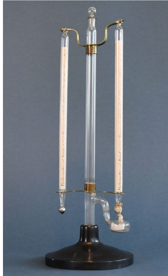
Fig. 8.5 Historical psychrometer according to August A. Greiner, Munich, 1850 (photo © Prof. Jürgen Baumüller)
