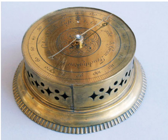
Fig. 8.1 Lambert's hygrometer from about 1772 (after [8.18]), using the torsion of catgut string. Translation of the German engraving: two graduations are 3 degrees of humidity within a cubic foot of air (photo © Freunde alter Wetterinstrumente, Riedlingen, Germany)
