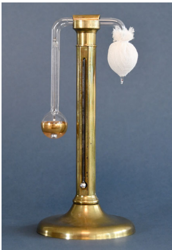
Fig. 8.7 Dewpoint hygrometer according to Daniell (photo © Prof. Jürgen Baumüller)
