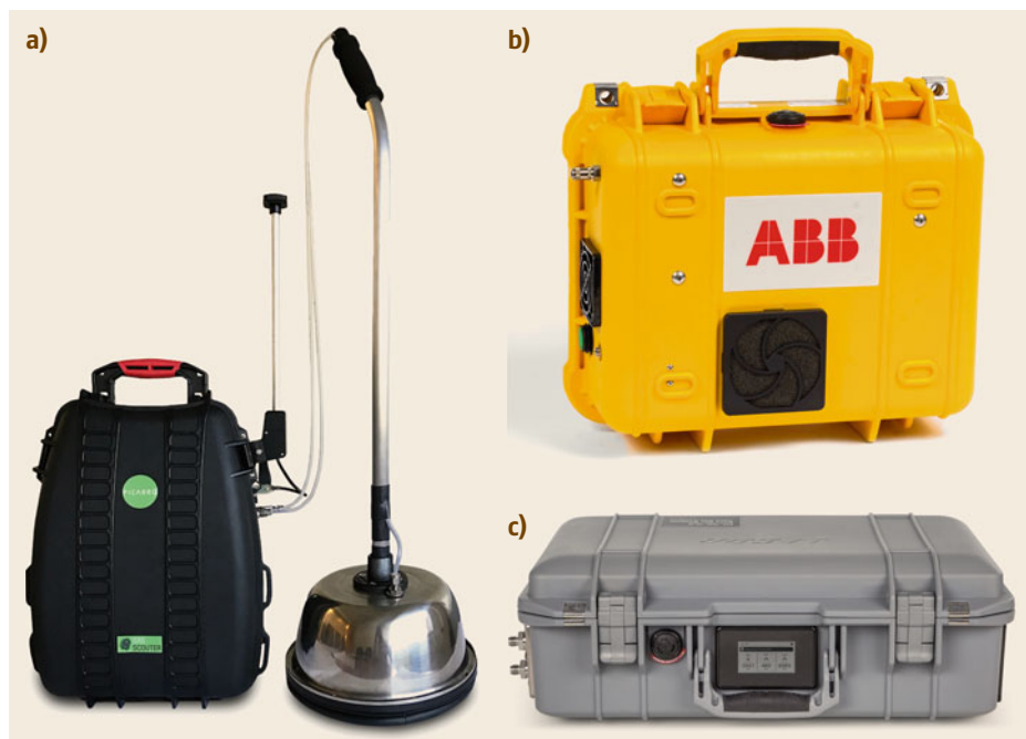
Fig. 60.6a–c Portable gas analyzers suitable for combined chamber-based measurements of \text{CH}_4 , \text{H}_2\text{O} and \text{CO}_2 . (a) GasScouter™ by Picarro, with attached soil chamber (diameter: 28 cm, V = 9340 \text{ cm}^3 ), which has the analytical unit contained in a backpack. (Reprinted with permission of Picarro Inc.) (b) Ultra-portable gas analyzer by Los Gatos Research ( 29.5 \times 34 \times 12 \text{ cm} ) (reprinted with permission from ABB). (c) Li-7810 by Li-Cor ( 51 \times 33 \times 18 \text{ cm} ) (image reprint with permission of LI-COR Biosciences)
