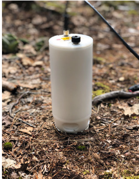
Fig. 60.8 Forced diffusion chamber eosFD by Eosense (diameter: 10.2 cm, 20 cm high) (reprinted with permission from Eosense Inc.)
