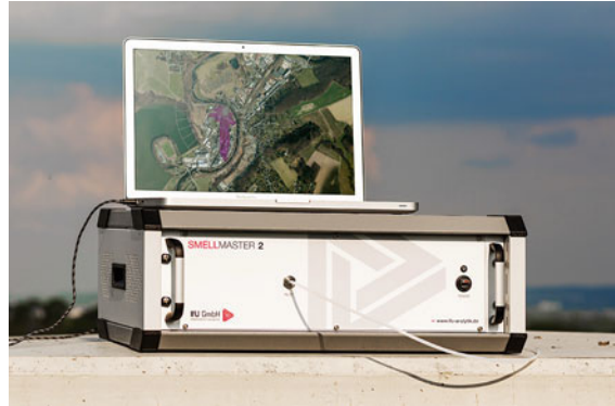
Fig. 21.2 Example for an IOMS based on ion mobility spectroscopy
