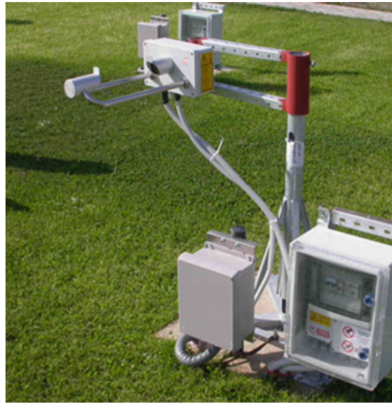
Fig. 12.7 Optical non-catching-type gauge (photo © Emanuele Vuerich)
