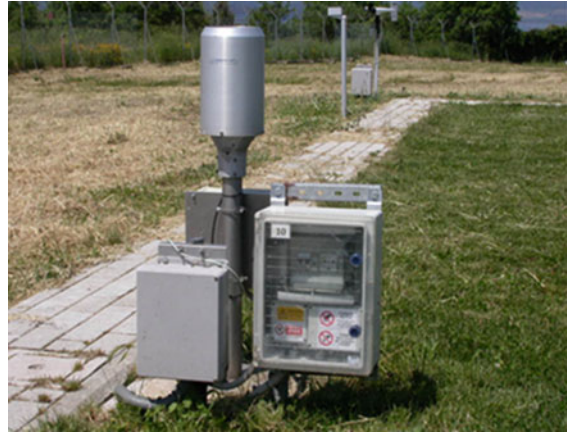
Fig. 12.5 Tipping-bucket gauge (photo © Emanuele Vuerich)
