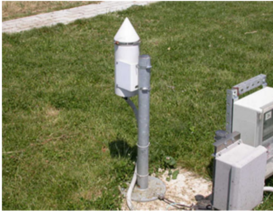
Fig. 12.8 Microwave precipitation gauge (photo © Emanuele Vuerich)
