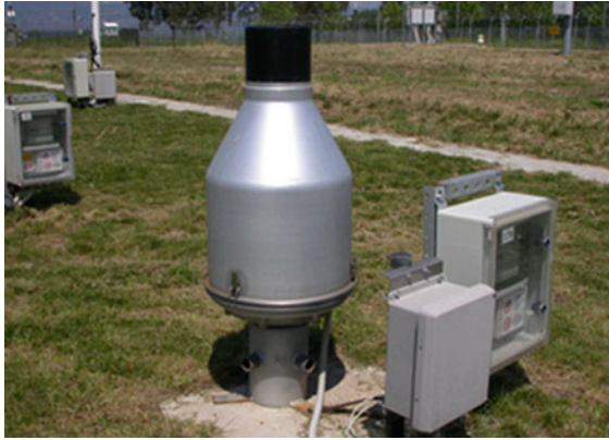
Fig. 12.6 Weighing gauge (photo © Emanuele Vuerich)
