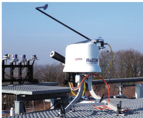
Fig. 11.36 RaZON+ (manufacturer: Kipp and Zonen B.V., the Netherlands): a solar tracker with pyr heliometer and shaded pyranometer measuring direct ( E ) and diffuse ( E_d\downarrow ) solar irradiance on the roof platform of the Meteorological Observatory Lindenberg – Richard-Abmann Observatory in Lindenberg, Germany (photo: K. Behrens)
