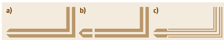
Fig. 9.9a–c Schematics of various Pitot tube configurations: (a) simple Pitot tube (sum of the dynamic and static pressures), (b) static tube (static pressure only), and (c) Pitot-static tube (Prandtl tube)
