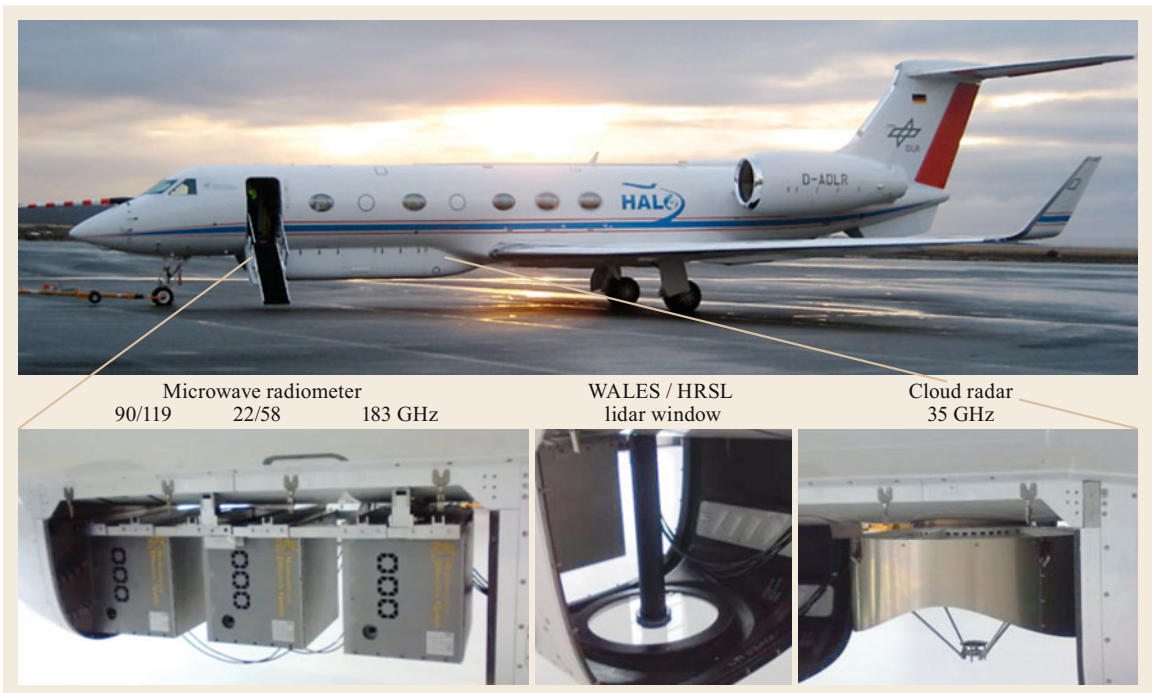
Fig. 39.13 Images showing the installation of the cloud radar antenna, including the clutter fence, lidar window, and microwave radiometers, in the HALO research aircraft belly pod (photos © M. Hagen)
