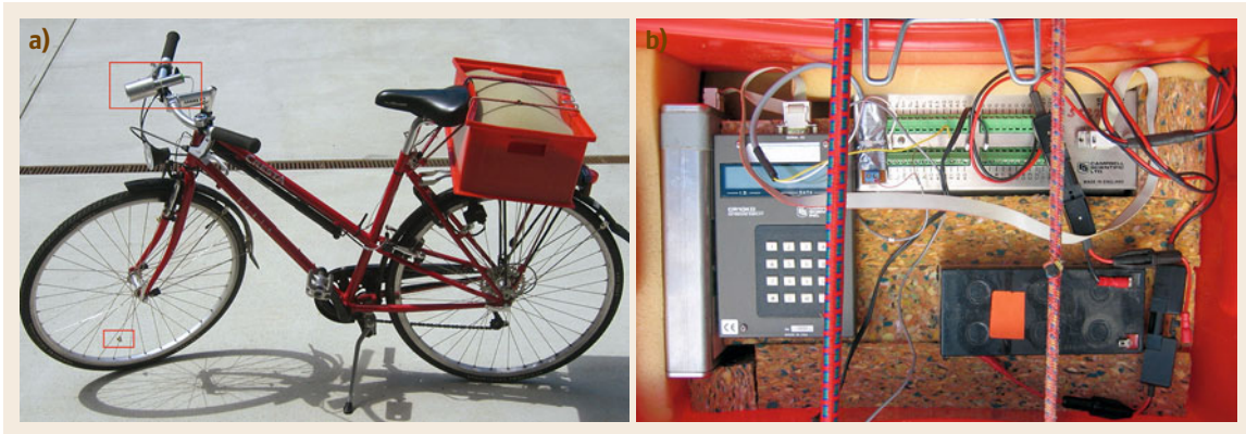
Fig. 50.6 (a) Bicycle unit with a thermistor (red frame) on the handlebar and (b) data storage box on the luggage rack (photo © E. Parlow)
