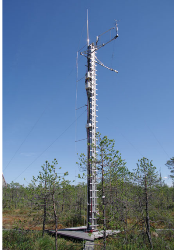
Fig. 6.11 A 10-m tower of box-type aluminum profile on a wooden platform in a swampy area in Central Siberia close to the Zotino Tall Tower Observatory (ZOTTO) (photo © Martin Hertel, MPI-BGC)
