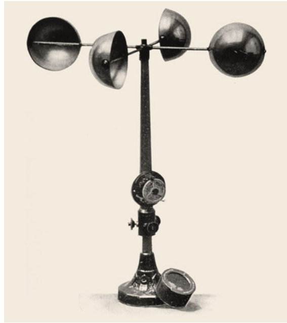
Fig. 9.3 Robinson’s cup anemometer from 1846 [9.15] (courtesy of the NOAA Photo Library, National Oceanic and Atmospheric Administration, Department of Commerce)
