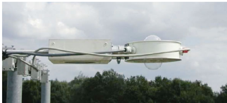
Fig. 11.14 Schulze radiation balance meter with blower (photo: K. Behrens)
