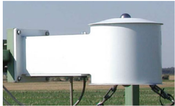
Fig. 11.32 An Eppley DDPIR net radiometer consisting of two PIR fit together in a case, which also contains the ventilation unit with heater (photo: K. Behrens)
