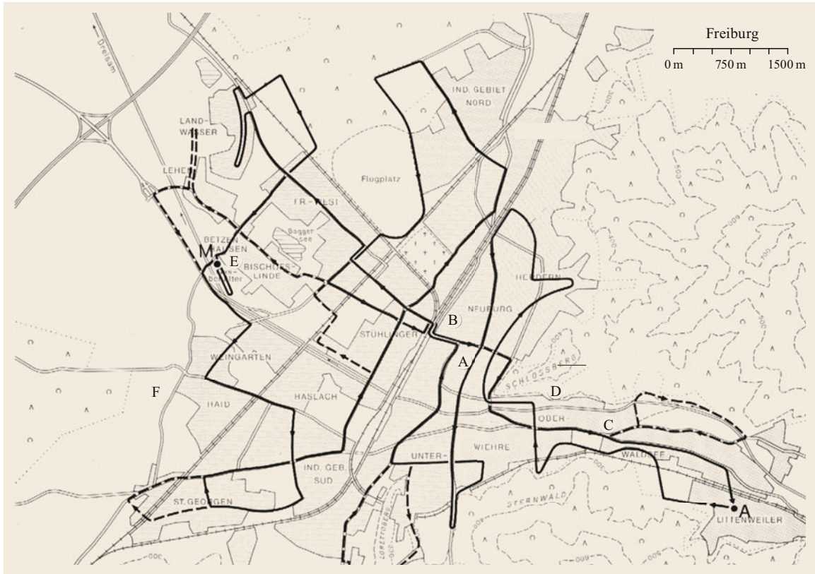
Fig. 50.2 Itinerary and locations of fixed weather screens (A–F) used in an urban climate study performed in the city of Freiburg. Measurements were initially taken at point A; all measurements were corrected for the base temperature at point E (after [50.8] with the permission of the Department of Physical Geography, University of Freiburg, Germany)
