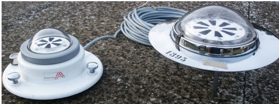
Fig. 11.11 Two star pyranometers from different generations: Left a modern one manufactured by Fa. Ph. Schenk, Wien and right a historical version from the 1930s (photo: K. Behrens)
