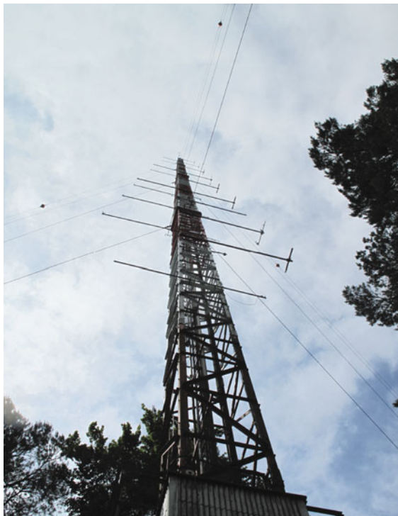
Fig. 6.19 The Karlsruhe KITcube tower, where anemometers are installed at the two prevailing wind directions to minimize the effect of wind distortion on the measurements (photo © Stephan Kraut, KIT)
