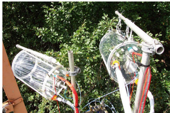
Fig. 59.1 Twin-cuvette system that can be used for measuring reactive trace gaseous fluxes under field and laboratory conditions (photo © Jürgen Kesselmeier)
