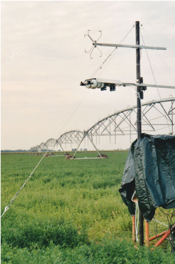
Fig. 56.1 DEC system with two grab sampling inlets and intermediate storage reservoirs (white cylindrical containers) in operation at an alfalfa field near Fort Morgan, Colorado, August 2000 (after [56.3, 4]). The DEC sampling unit is positioned 0.6 m below the sonic anemometer at 3.2 m (photo © Janne Rinne)
