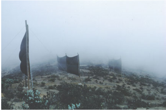
Fig. 53.1 A portion of the array of large fog collectors used in the El Tofo project in Chile during the late 1980s and 1990s (photo © Robert S. Schemenauer 2020; all rights reserved)
