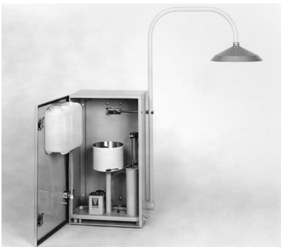
Fig. 57.2 Evaporimeter developed by Czeratzki (photo © Adolf Thies GmbH & Co. KG, Göttingen, Germany)
