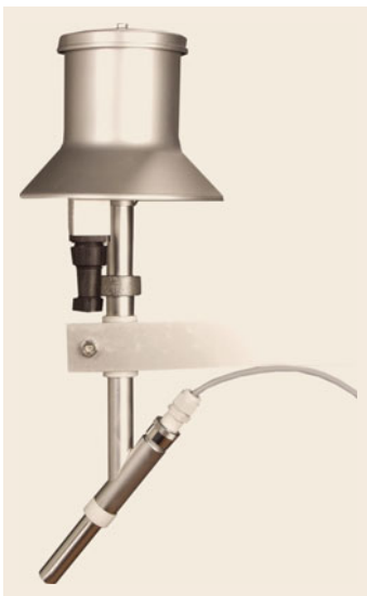
Fig. 7.16 Assmann aspirated psychrometer with one sensor (a resistance thermometer), ventilation, and a double-tube radiation shield (photo © Theodor Friedrichs & Co., Schenefeld, Germany, 2018)
