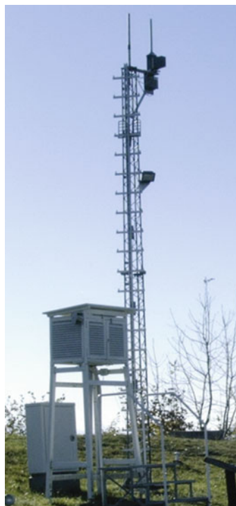
Fig. 6.2 Instrument shelter and mast for wind measurements at the Hohenpeißenberg Meteorological Observatory (photo (enlarged detail) © Christoph Radtke)
