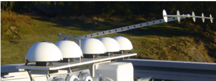
Fig. 11.41 Shaded pyrometers of PIR and CG4 type of the WISG, assembled in a ventilation and heating unit at a Sun tracker during IPgC-II on the roof of PMOD/WRC Davos in September/October 2015 (photo: K. Behrens)
