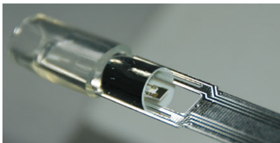
Fig. 46.4 Humidity sensor of the Chang Feng CF-06-A radiosonde underneath its protective cap
