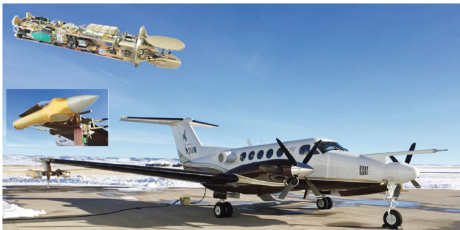
Fig. 39.15 The Ka-Band Precipitation Radar mounted on the Wyoming King Air research aircraft. The radar is mounted on the right wing (see the inset showing a close-up image of the wing tip). The inset in the top left corner shows the internal components of the radar, including the two flat-plate antennas (photos © A. Pazmany)
