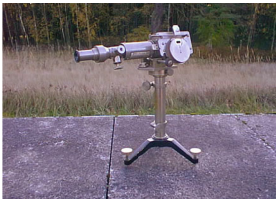
Fig. 11.8 Michelson–Marten pyrheliometer with the rectangular entrance, that can be seen in the photo (photo: K. Behrens)
