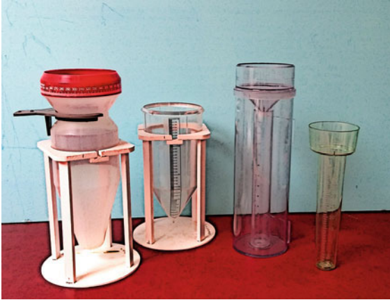
Fig. 12.4 Plastic storage gauges developed for agricultural purposes (WMO-METAGRI project; photo © Mattia Stagnaro)
