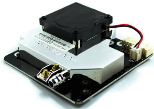
Fig. 44.5 The $20-fine dust sensor SDS011 is (among other low-cost sensors of similar design) used in different crowdsensing campaigns around the world, such as the luftdaten.info project of the Open Knowledge Foundation Germany (image taken from Wikimedia under CC0 1.0 Universal license)
