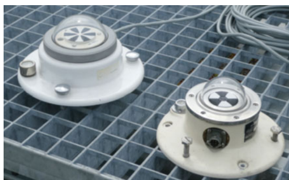
Fig. 11.30 Star pyranometer (left) and black-and-white pyranometer (right) (photo: K. Behrens)
