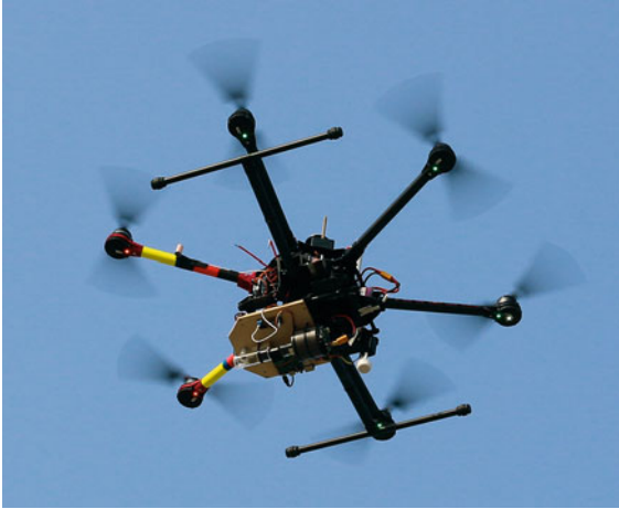
Fig. 49.1 Example of a multicopter research UAS. This system is equipped with a particle and pollen trap (photo © Jens Bange, University of Tübingen)
