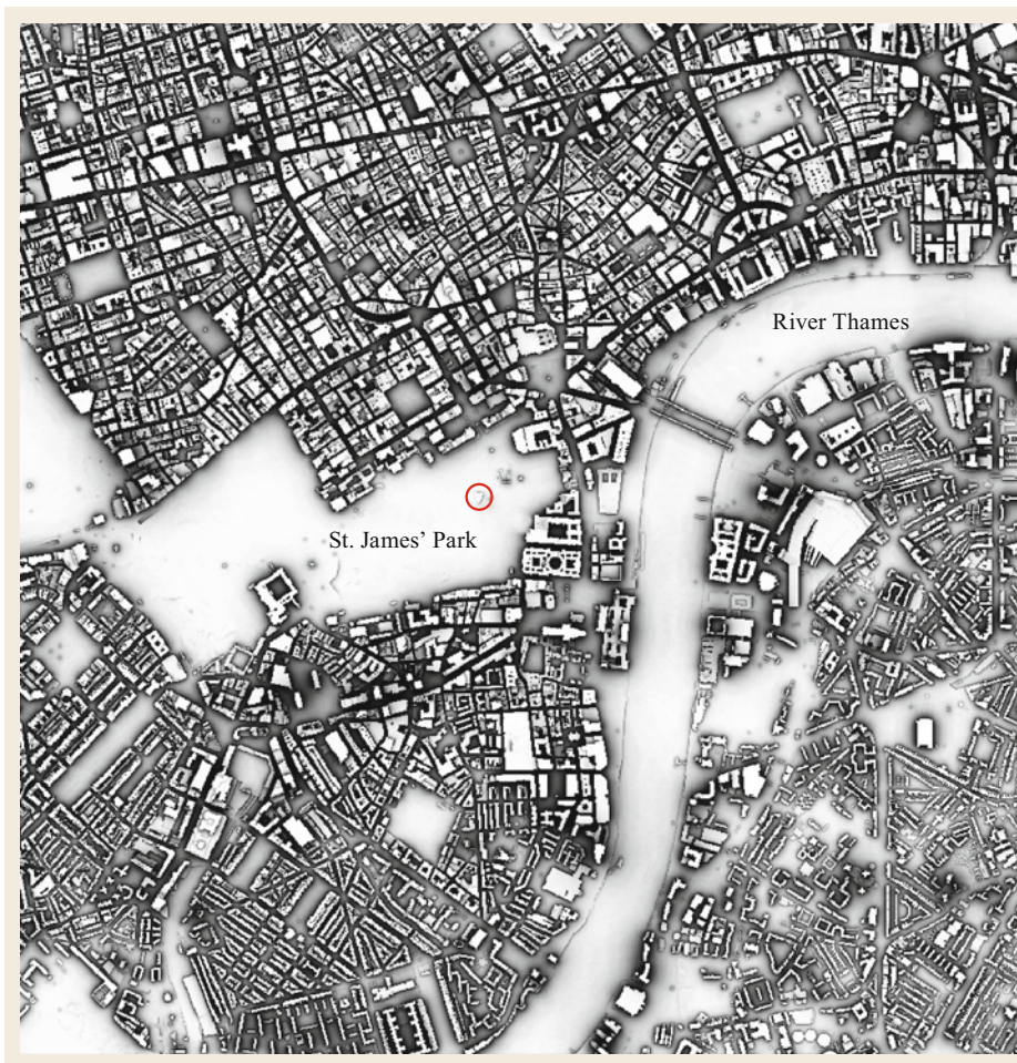
Fig. 52.6 Location of a weather station in St James' Park (red circle) London, which has much lower sky-view factor (SVF) (white) than the surrounding built-up areas. The streets are black (lower SVF) and the roofs white (higher SVF). SVF at 4 m-resolution modified (after [52.146])
