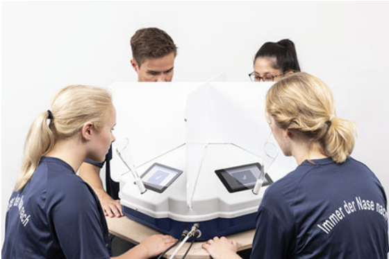
Fig. 21.1 Example for an olfactometer with panel members during a measurement (photo courtesy Olfasense)
