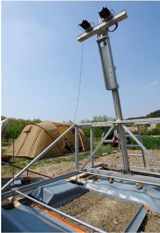
Fig. 61.7 Using stereo photography for quantifying surface storage of water
