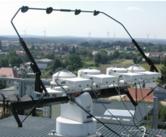
Fig. 11.31 Two Eppley PIRs ( center ) flanked by two Kipp and Zonen CG4 pyrgeometers within a ventilation unit on an Eppley SMT tracker modified at Meteorological Observatory Lindenberg – Richard-Aßmann Observatory for the use of four instruments to shade and protect the pyrgeometer domes for additional solar beam heating (photo: K. Behrens)
