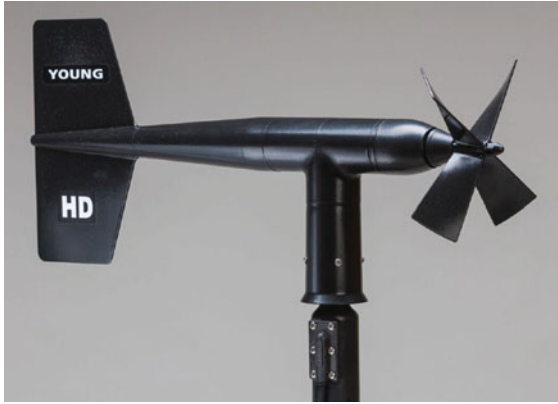
Fig. 9.16 Combination of a propeller anemometer with a mechanical wind vane, also called a skyvane (photo © R.M. Young Company/GWU-Umwelttechnik GmbH, Erftstadt, Germany)
