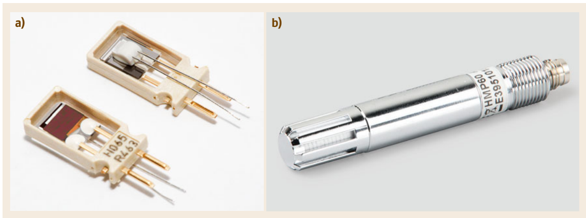
Fig. 8.17a,b Capacitive humidity sensor: (a) sensor element ( lower : view of the temperature sensor, upper : view of the humidity sensor); (b) housing of the sensor with filter screen and electronic tube (photos © Vaisala Oyj., Vantaa, Finland)
