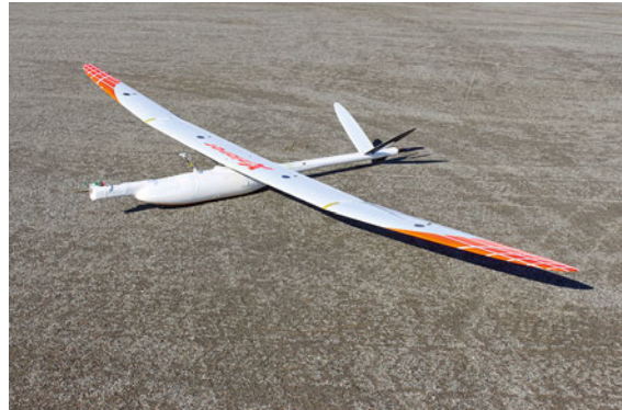
Fig. 49.3 Example of a light class UAS: the Multipurpose Airborne Sensor Carrier MASC-3, designed and operated by the University of Tübingen, Germany (photo © B. Altstädter)
