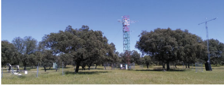
Fig. 6.28 A measurement setup near Majadas, Spain with a subcanopy eddy-covariance system on tripod ( left ), a 15-m walk-up tower with eddy-covariance system and meteorological measurements ( center ), and a 10-m triangular mast with rotatable arm for spectral radiative measurements ( right ) (photo © Tiana Hammer, MPI-BGC)
