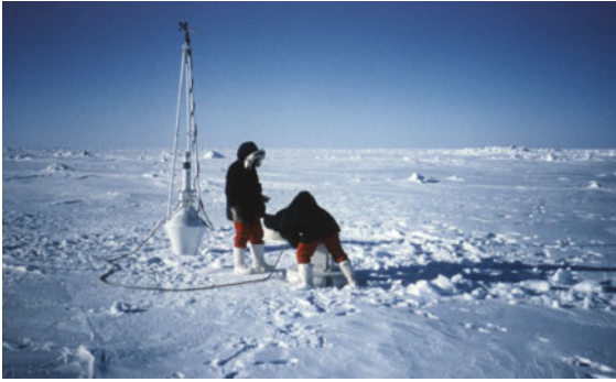
Fig. 6.21 An antarctic sea ice buoy deployed during the 1989 Winter Weddell Gyre Study by Alfred Wegener Institute Bremerhaven/Univ. Hannover. It takes meteorological observations with a propeller/wind vane anemometer on a 3-m tripod, air pressure, air temperature, and ocean mixed-layer temperatures with a 200-m-long thermistor chain beneath the 2-m-thick ice flow, and sea ice temperature profiles with a thermistor rod (photo © D. Engelbart)
