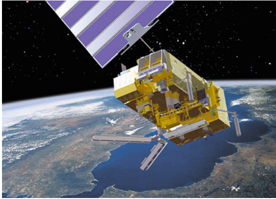
Fig. 42.1 The MetOp-C satellite is the newest of the first generation of Europe’s EUMETSAT Polar System series (following Metop-A and -B) that orbit at 817 km (© ESA)
