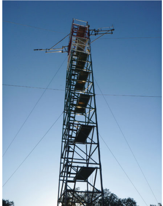
Fig. 6.8 A 15-m walk-up tower near Majadas (Spain) with eddy-covariance system and instruments for radiation and standard meteorological measurements (photo © Martin Hertel, MPI-BGC)
