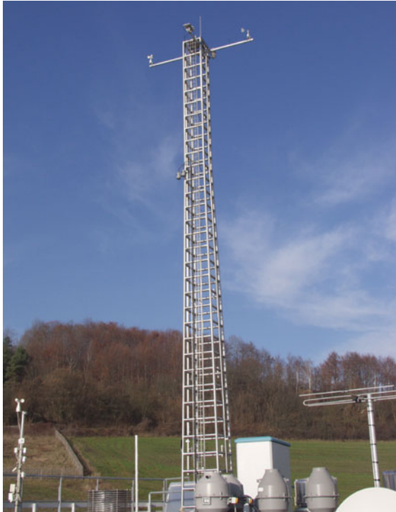
Fig. 6.6 The 10-m-high, stainless-steel, and self-supporting mast on the roof of the Max Planck Institute for Biogeochemistry in Jena, Germany (photo © Olaf Kolle, MPI-BGC)
