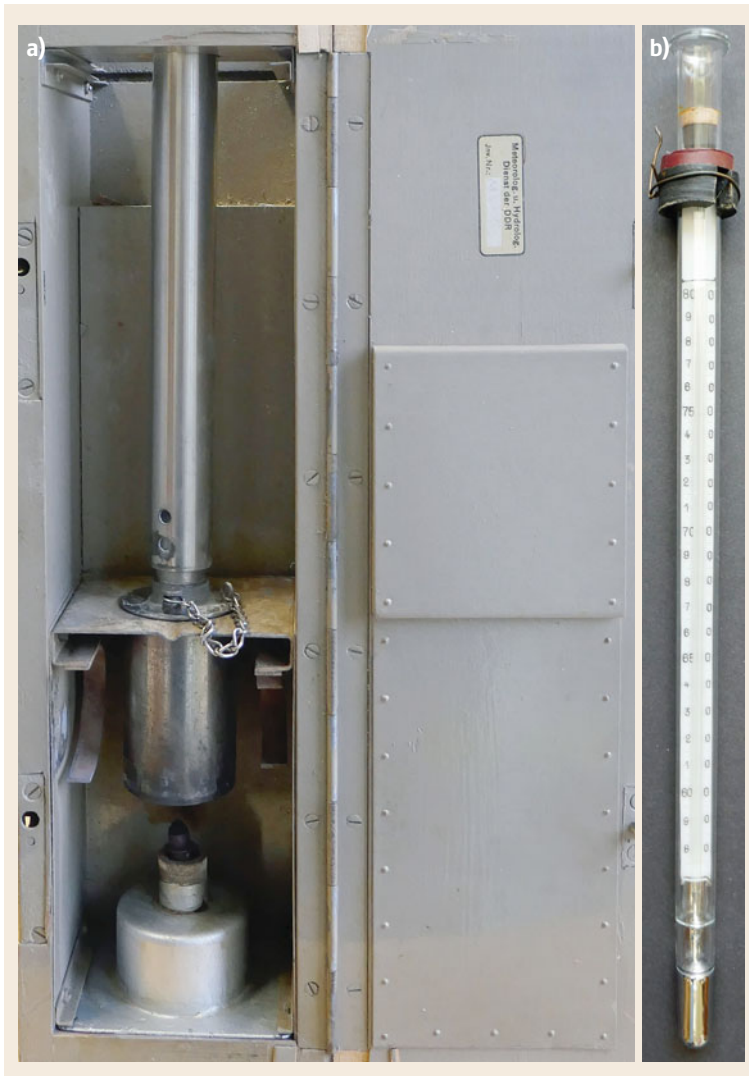
Fig. 10.15 (a) Hypsometer for balloon investigations with a heater, boiler, and tube for steam; (b) hypsometer thermometer with an enlarged temperature range from 60 to 80 mm Hg (approximately up to heights of 2 km). Photo © Weather Museum, Lindenberg, Germany
