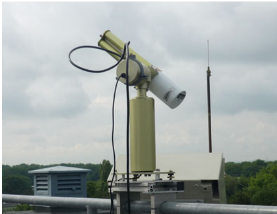
Fig. 29.3 Photo of a sun photometer at the Jülich Observatory for Cloud Evolution (JOYCE) (photo © Birger Bohn)
