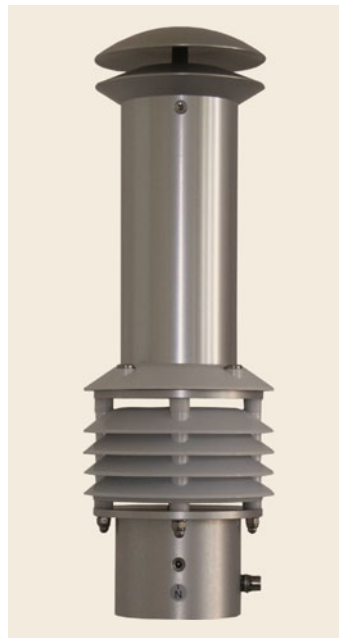
Fig. 9.19 Thermal anemometer (top part) combined with a temperature screen (photo © Lambrecht Meteo GmbH, Göttingen, Germany)
