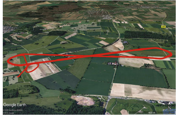
Fig. 49.12 Repeated legs for maximum significance or temporal development (after [49.38] © A. Rautenberg et al. 2018, Creative Common Attribution 4.0 License)
