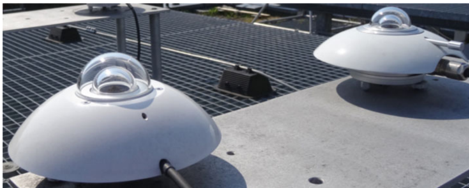
Fig. 11.27 Two different pyranometers of black thermopile type: SR12 (left) and SR22 (right), here without ventilation unit (manufacturer: Hukseflux Thermal Sensors B.V., the Netherlands, photo: K. Behrens)
