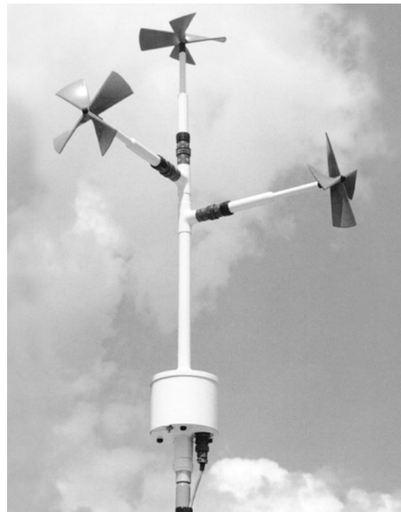
Fig. 9.13 The Gill 27005T UVW three-component propeller anemometer (photo © R.M. Young Company/GWU-Umwelttechnik GmbH, Erfstadt, Germany)
