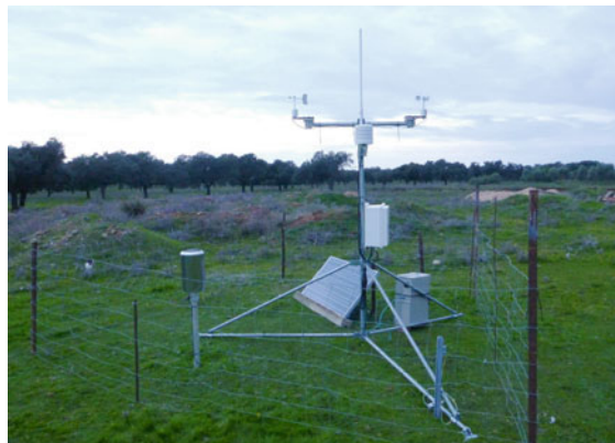
Fig. 6.3 A temporary weather station on a tripod with instruments for wind velocity, wind direction, air temperature, and humidity as well as a precipitation gauge on a simple pole (photo © Olaf Kolle, MPI-BGC)
