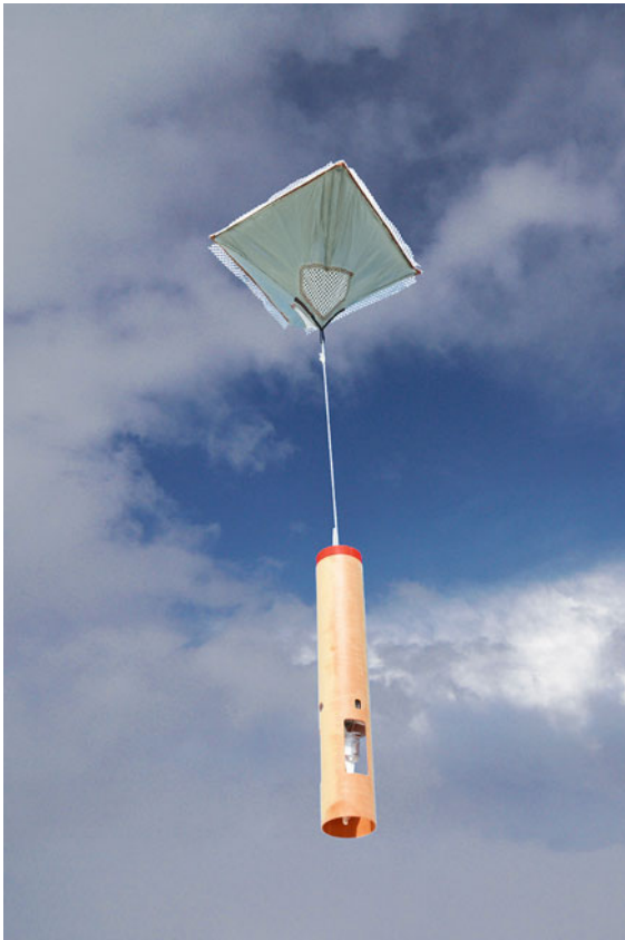
Fig. 46.7 Image of the NCAR NRD41 dropsonde
