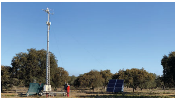
Fig. 6.13 A mobile mast with a maximum height of 25 m in the Spanish Dehesa (photo © Olaf Kolle, MPI-BGC)
