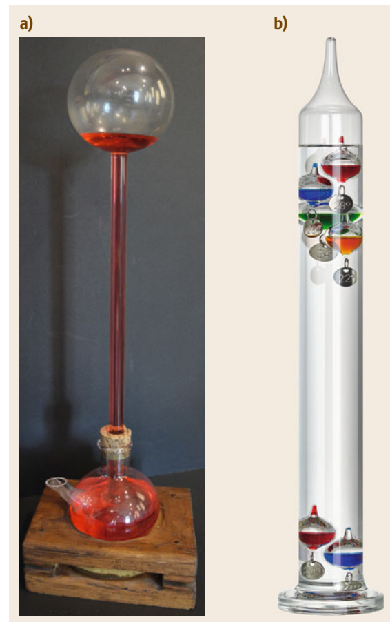
Fig. 7.1 (a) Reconstruction of Galileo's thermoscope (photo © Deutsches Thermometermuseum Geraberg, Germany; the original is on display at the Museo Galileo in Florence). (b) Galileo thermometer (photo courtesy of TFA Dostmann, Wertheim, Germany)
