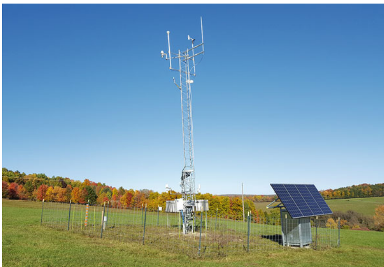
Fig. 45.1 A typical mesonet weather station equipped with a 9.1 m ( \approx 30 ft) tower, communications, power, datalogger, and sensors (photo: courtesy of the New York State Mesonet at the University at Albany)
