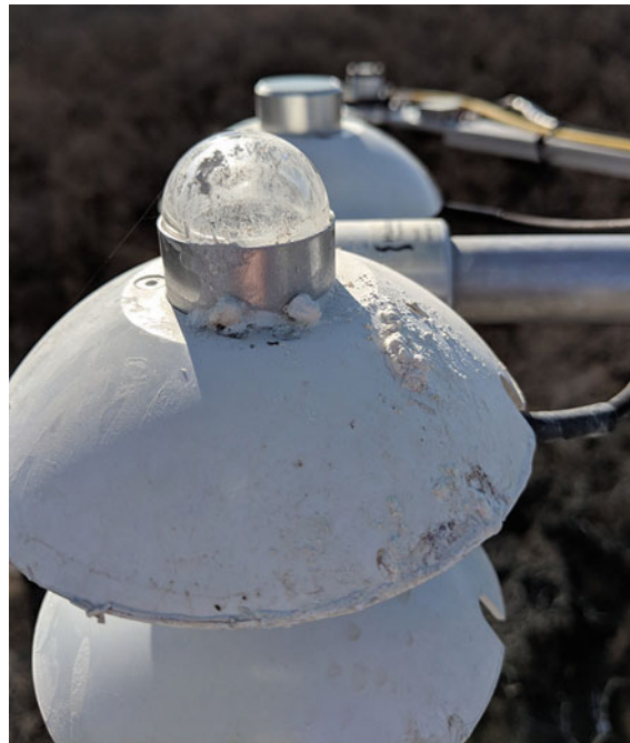
Fig. 3.2 Bird fouling on a radiation sensor at the NEON Lyndon B. Johnson National Grasslands site in Texas, USA (photo © Gary Henson, National Ecological Observatory Network, USA)
