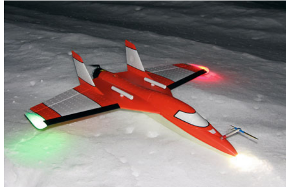
Fig. 49.2 Example of a very light class UAS: the SUMO, designed and operated by the University of Bergen Norway (after [49.12] photo is not included in [49.12])
