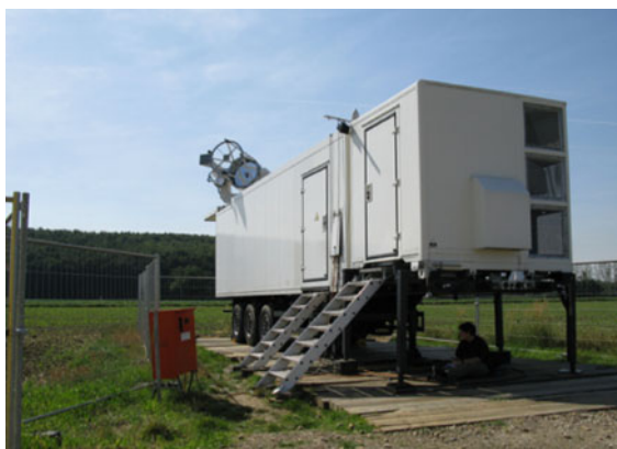
Fig. 26.3 The current state-of-the-art high-power ground-based water vapor DIAL is represented by the UHOH 3-D-scanning WVDIAL. The instrument is housed inside a mobile trailer. The 80-cm 3-D scanner can be seen protruding out of the top left of the trailer (photo by Andreas Behrendt; used with permission)
