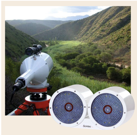
Fig. 34.10 The BLS-900 transmitter and receiver units (courtesy of Scintec AG; background photo kindly provided by C. Jarman – South Africa)
