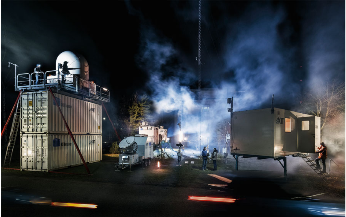
Fig. 47.4 A composite photo of KITcube in operation. From left to right: X-band radar, cloud radar, ceilometer, micro rain radar, disdrometers, two Doppler radars, 30 m tower, energy-balance station, and office container (photo © Markus Breig/KIT, used with permission)
