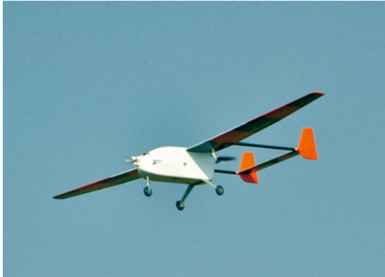
Fig. 49.4 Example of a medium class UAS: ALADINA, designed and operated by the TU Braunschweig, Germany (photo after [49.17], © B.Altstädter et al. 2015, Creative Commons Attribution 3.0 License)
