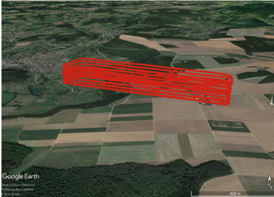
Fig. 49.14 Stacked race-track patterns are well suited for wind-energy research (after [49.38] © A. Rautenberg et al. 2018, Creative Common Attribution 4.0 License)
