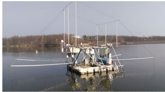
Fig. 6.24 A Technical University of Dresden measurement float with eddy-covariance sensors on a reservoir during the project Greenhouse gas emissions from reservoirs (TREGATA) (photo © Dr. Uwe Spank)
