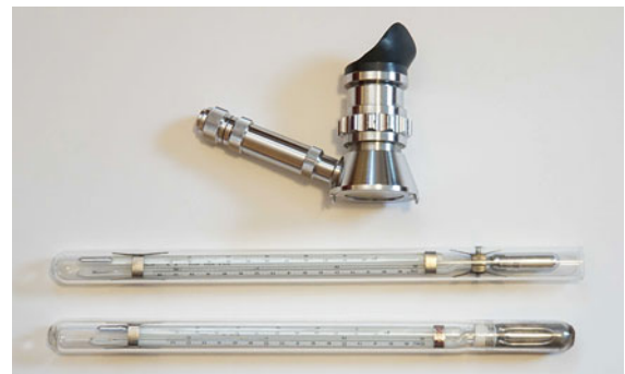
Fig. 62.1 Open and closed reversing mercury thermometers ( middle and bottom ) and the reading magnifier ( top ) (photo © V. Mohrholz)
