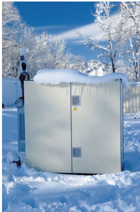
Fig. 26.4 The current state-of-the-art low-power ground-based water vapor DIAL is represented by the micropulse DIAL (MPD) developed by NCAR and Montana State University. Photo taken March 2016, Boulder CO, USA (photo by Rich Erickson; used with permission)
