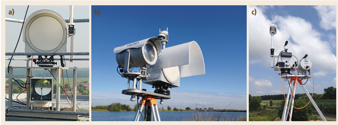
Fig. 34.11a–c The RPG MWSC-160 combined with different LAS systems; (a) with a WURMAQ LAS at the tower at Lindenberg Meteorological Observatory – Richard-Aßmann-Observatory, (b,c) with a Kipp & Zonen LAS MkII system (photos courtesy of DWD and Kipp & Zonen B.V., respectively)
