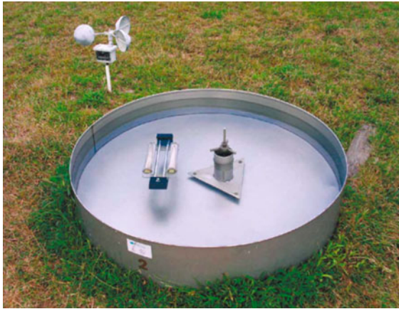
Fig. 57.6 Class A pan with a cylinder to measure the water level; temperature and wind sensors are also present (photo provided courtesy of the Hong Kong Observatory of HKSAR)
