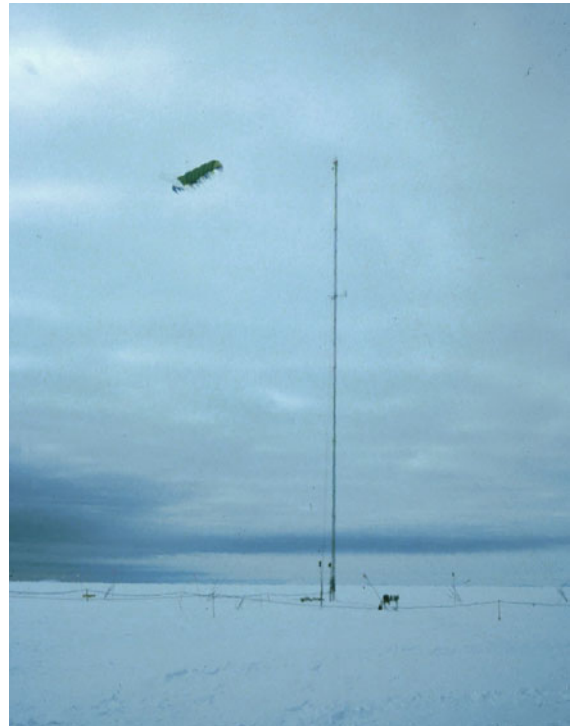
Fig. 47.2 Obtaining integrated vertical profiles with a 45 m high mast and a kite-mounted tethered sonde at the German Antarctic Neumayer Station in 1983 (after [47.55] photo © Ch. Kottmeier)
