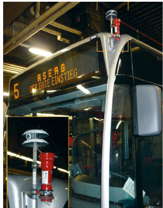
Fig. 50.5 Combined temperature sensor and GNSS logger mounted on a public bus (after [50.39] © the authors, CC Attribution 3.0 License)
