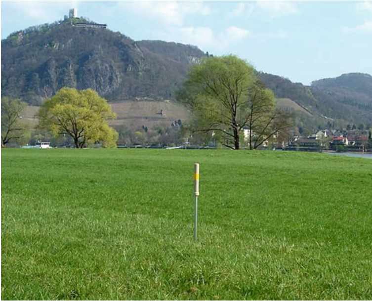
Fig. 15.1 A probe of the German gamma dose rate network at a representative measuring site
