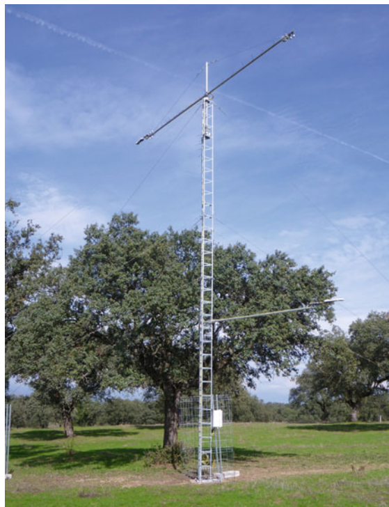
Fig. 6.14 A 10-m mast with rotatable arm on top (photo © Olaf Kolle, MPI-BGC)
