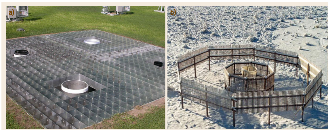
Fig. 12.12a,b The realization of the reference rain gauge pit at Vigna di Valle, Italy (2007) (WMO field intercomparison of rainfall intensity gauges, 2009; photo © Emanuele Vuerich) (a) and a DFIR equipped with a Geonor T-200B weighing gauge located at the experimental site in Marshall (Colorado) (b) (after [12.62] © American Meteorological Society. Used with permission)
