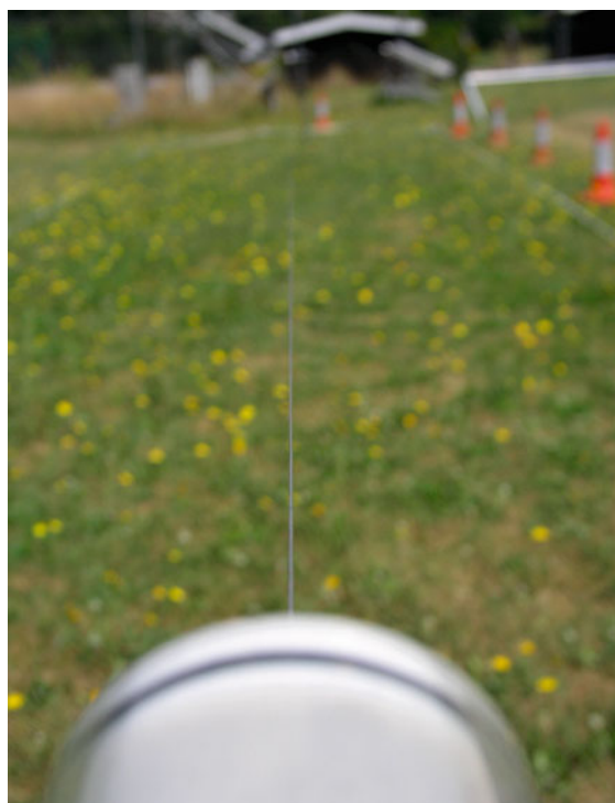
Fig. 14.5 Passive wire apparatus showing the thin and long sensing wire emerging from a PTFE insulator. (photo: A.J. Bennett)
