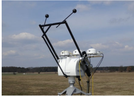
Fig. 11.38 Fully equipped solar tracker (solar tracker and radiation instruments: Kipp and Zonen B.V., the Netherlands; ventilation and heating units: Fa. Eigenbrodt GmbH and Co KG, Germany) at the Boundary Layer Measuring Field Falkenberg of the Meteorological Observatory Lindenberg – Richard-Aßmann Observatory (photo: K. Behrens)
