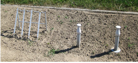
Fig. 61.22 Measurement plot for soil temperatures according to World Meteorological Organization (WMO) regulations (after [61.104] photo © T. Foken)
