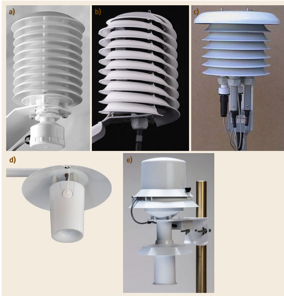
Fig. 7.15a–e A selection of nonventilated ( a,b ) and ventilated ( c–e ) temperature screens: ( a ) screen developed by Gill (model 41003; photo © R. M. Young/GWU Umwelttechnik GmbH, Erfstadt, Germany); ( b ) naturally aspirated helical radiation screen (photo © baranidesign, Bratislava, Slovakia); ( c ) ventilated screen of the German Meteorological Service with four sensors (photo © Eigenbrodt GmbH & Co. KG, Königsmoor, Germany); ( d ) aspirated screen (photo © Apogee Instruments, Logan, UT, USA); ( e ) ventilated temperature screen (model 43502; photo © R. M. Young/GWU Umwelttechnik GmbH, Erfstadt, Germany)
