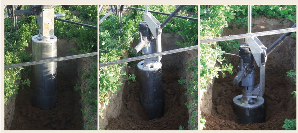
Fig. 58.3 Excavation of a monolith intended for a small lysimeter in three steps (photo © S. Reth)
