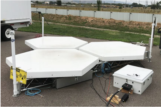
Fig. 31.14 The NCAR Modular Profiler is an example of a spaced antenna radar. This 449 MHz radar uses a number of hexagonal antennas—three are employed in the boundary-layer configuration shown, but the system can also be deployed in a seven-panel configuration for higher altitude measurements. All of the antenna panels are used for transmission and each panel has its own receiver system
