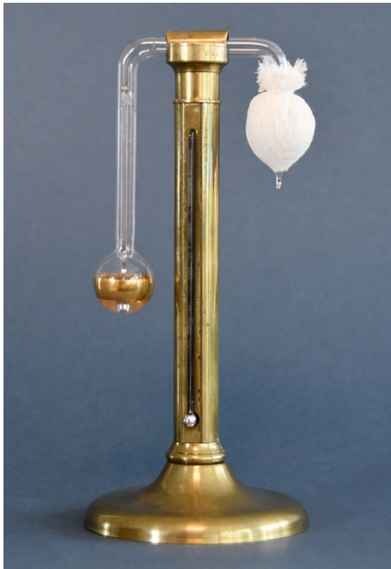
Fig. 8.7 Dewpoint hygrometer according to Daniell (photo © Prof. Jürgen Baumüller)
