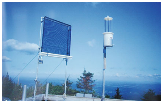
Fig. 53.4 The 1 m 2 SFC ( on the left ) and the Environment Canada version of the ASRC collector (after [53.66]) ( on the right ). The photo was taken during the Chemistry of High Elevation Fog project in southern Québec, Canada (photo © Robert S. Schemenauer 2020; all rights reserved)
