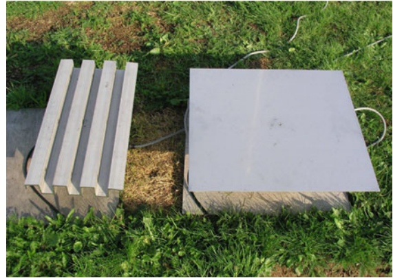
Fig. 14.9 Measurement of the conduction and displacement current densities using the combined two electrodes of different geometry in a GDACCS instrument. (photo: A.J. Bennett)
