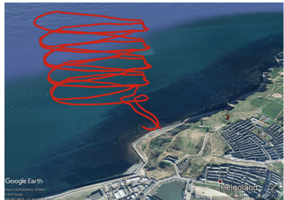
Fig. 49.13 A combination of legs with slant flights gives a spatial data set of atmospheric quantities (after [49.38] © A. Rautenberg et al. 2018, Creative Common Attribution 4.0 License)
