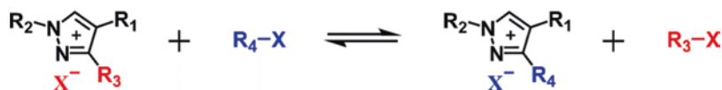
Fig. 7.16 Transalkylation of triazolium salts between 1,2,3-triazolium salts and alkyl halide. Reproduced with permission from Obadia et al. (2015)
