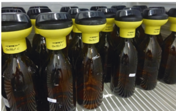
Fig. 8.4 Measuring heads used to monitor O 2 production
