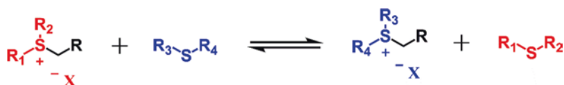
Fig. 7.18 Transalkylation of trialkylsulfonium salts between trialkylsulfonium salts and thioethers. Reproduced with permission from Hendriks et al. (2017)
