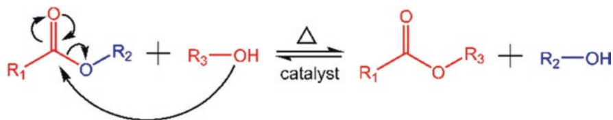
Fig. 7.2 Thermal-induced catalytic transesterification. Reproduced with permission from Otera (1993)
