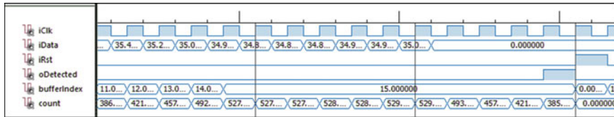
Fig. 11.5 Fall detector emulation. In it we can see how a fall is detected and how it restarts the operation when the reset button is pressed
