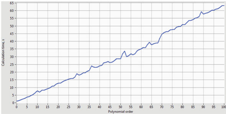
Fig. 11 The dependence of calculation time on the number of polynomials (for representation of 2D sine function with dimension 1000 \times 1000 )
