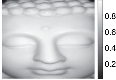
Fig. 2.7 The irradiance image I \in [0, 1] approximated based on (2.44) corresponded to the Buddha bust made from matte materials shown in Fig. 2.4. The maximum irradiance value appears almost on the tip of the nose and is used as the boundary point to both methods Tankus et al. [54] and Yuen et al. [66] and in the direction of reconstructing a 3D model of the bust
