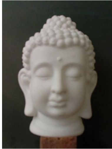
Fig. 2.4 The Buddha bust with a matte surface being captured by an endoscopic camera PiAEK equipped with 8 high-brightness light LEDs integrated with the endoscope. The camera has a small focal length of approximately 4 millimeter. The bust was located at a distance less than 5 cm while being captured in an intentionally darkened room. The motivation to capture the bust in a very short distance was to make it reasonable to employ the perspective projection
