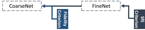
Fig. 3.6 Criterion flow. Gradients from both loss criteria are propagated back to CoarseNet
