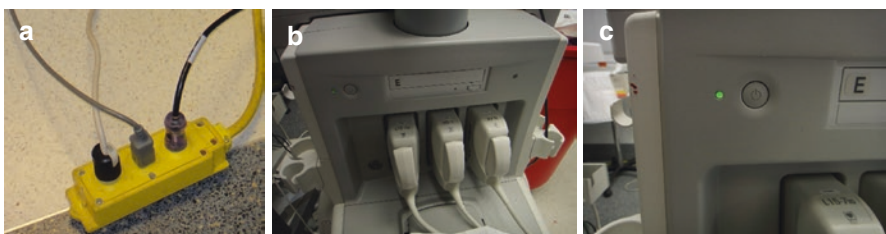
Fig. 12.1 Pictures of Left: Plug in the power cord Middle: Attach the echo probe to the machine Right: Press the power button to turn the machine on
