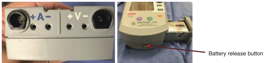
Fig. 32.7 Image showing Left : pacemaker connecting part Right : Battery housing
