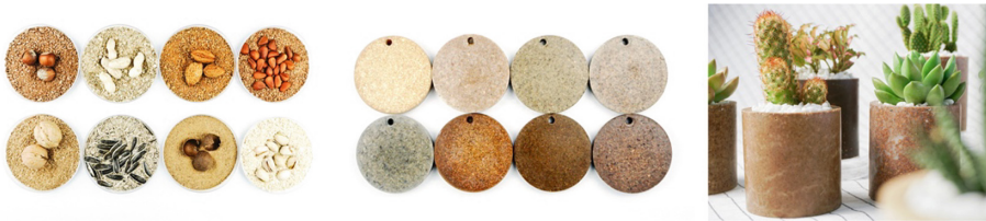
Fig. 1. Nut shell - bioplastic. Design by Beijing Institute of Fashion Technology, Innovative Materials Research Centre, 2018
