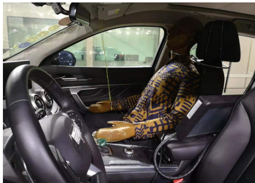
Fig. 2. Measurement of the equivalent space temperature in the vehicle by using the warm manikin
