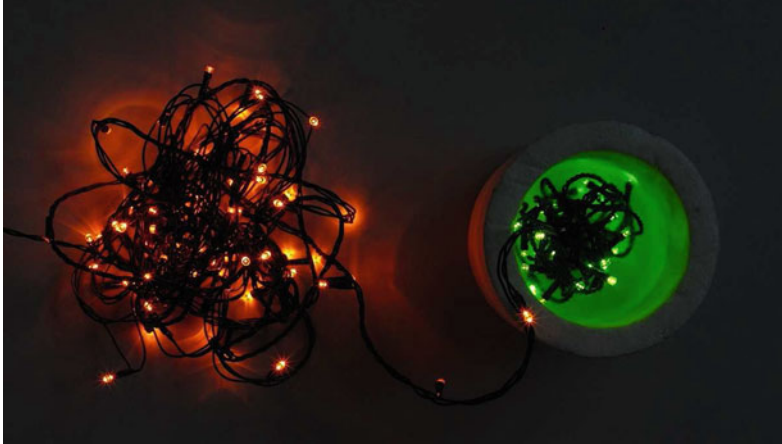
Fig. 6.28 LED chain with part at room temperature (left) and a part in a dewar filled with liquid nitrogen (right)
