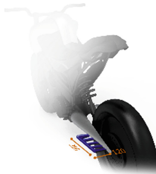
Fig. 5. Motorcycle with footrest design
