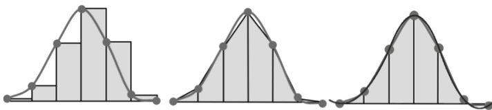
Fig. 1. Numerical integration methods (f.l.t.r.): R, T and S (dark grey: interpolated function, light grey: approximated area, circles: discrete loading data)
