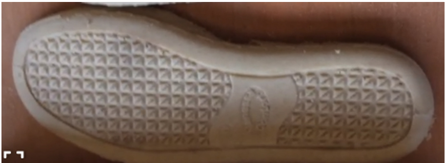
Fig. 1. The right sole developed with biodegradable material with outsole pattern designed with 2 mm square shapes and dashed diagonal lines.
