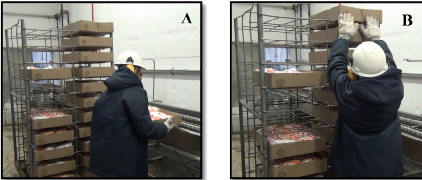
Fig. 1. Description of manual handling task (A – picking up the box on the conveyor belt; B – putting the box on the trolley).
