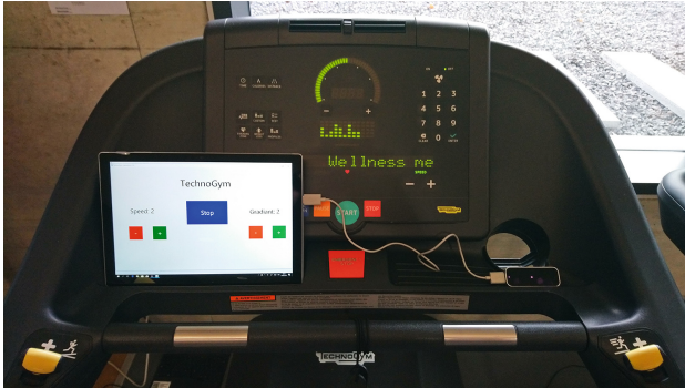
Fig. 1. On the left the tactile interface on a tablet and on the right the Leap Motion, everything is on the treadmill that will be used by the runner.
