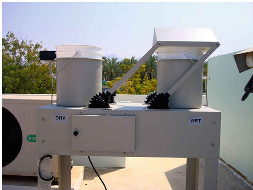
Fig. 3 An Automatic Andresen dry and wet acid rain sampler installed at a coastal station of UAE
